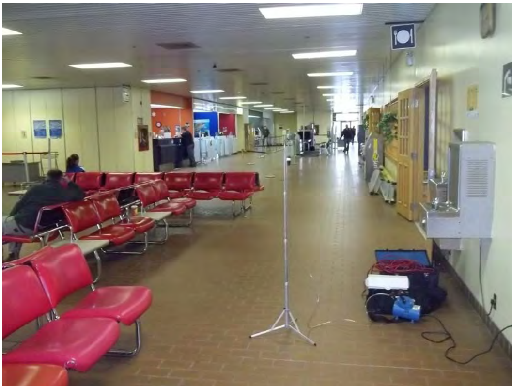
Photo 2: View, showing air sampling set-up at sample location AS-09 (Air Terminal Building, 1st level, Public Waiting Area).
