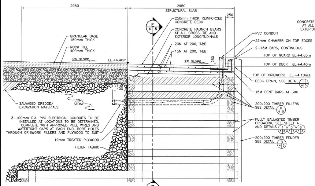
REINFORCED CONCRETE DECK DETAIL
