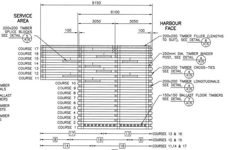
CRIB No.1 END CELL ELEVATION (CRIB No.3 OPPOSITE HAND)
