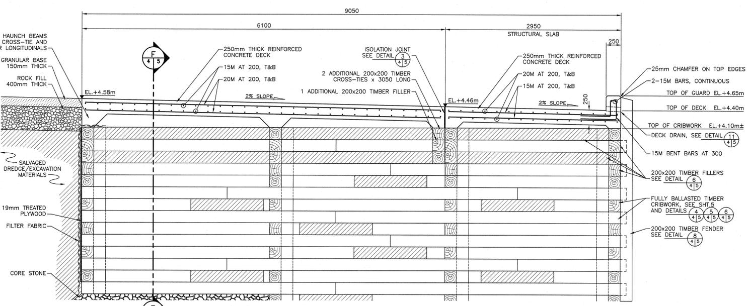
REINFORCED CONCRETE DECK DETAIL
