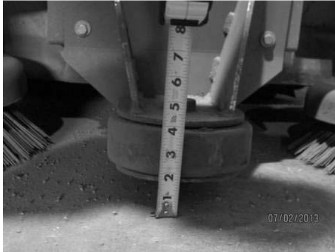
Figure 2: Guide Wheel on Existing Vehicle
