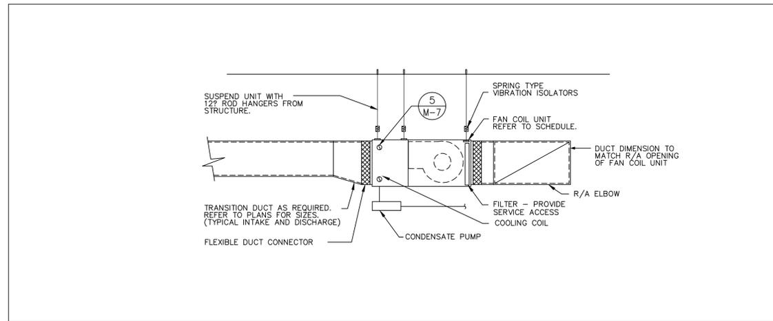
2 FAN COIL UNIT INSTALLATION DETAIL
