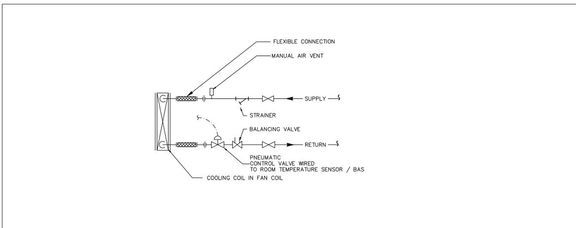
5 FAN COIL PIPING DETAIL
