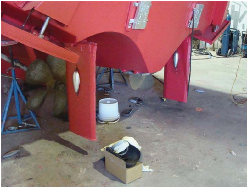
Figure E-01-Fig. 2 Rudders with view of rudder stocks.
