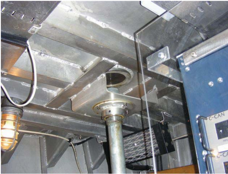
Figure E-01-Fig. 1 Extended spindle for emergency steering.
