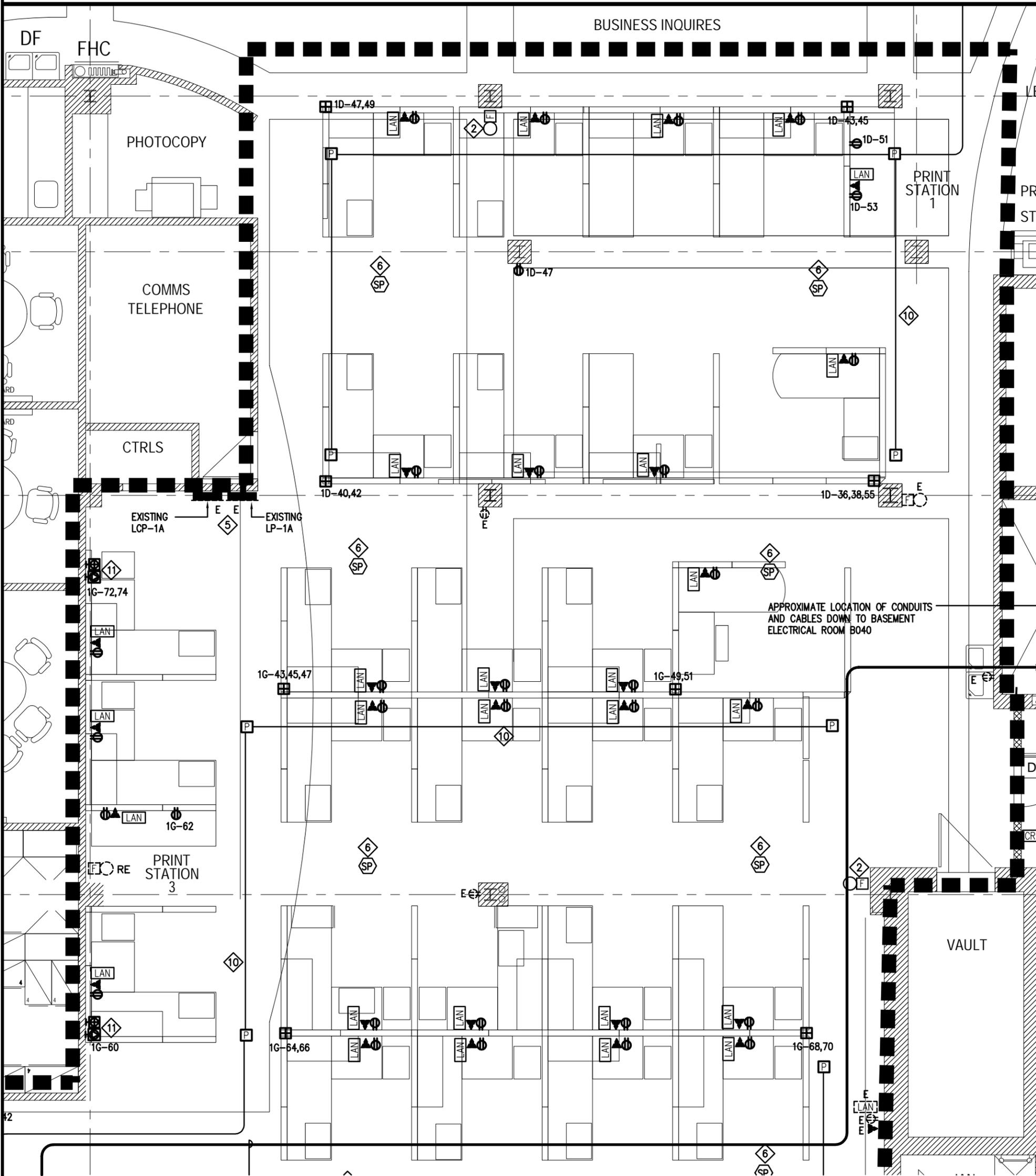
11 POWER AND SYSTEMS BASE FEED WHIP CONNECTION. MAKE PROVISIONS AND ALLOW FOR WALL MOUNTED BASE FEED FURNITURE WHIP CONNECTIONS COMPLETE WITH RECESSED PULL BOXES; COVER PLATE WITH CENTER CONNECTION AND FLEXIBLE CONDUIT WITH 90 DEGREE CONNECTION TO DEVICES THROUGH THE SYSTEM FURNITURE ASSEMBLY. ALLOW FOR ENOUGH WIRE SLACK TO REACH WORKSTATION DEVICES. CO-ORDINATE EXACT LOCATIONS FOR EACH OF THESE CONNECTIONS WITH SYSTEM FURNITURE SUPPLIER/INSTALLER PRIOR TO ROUGHING-IN.
