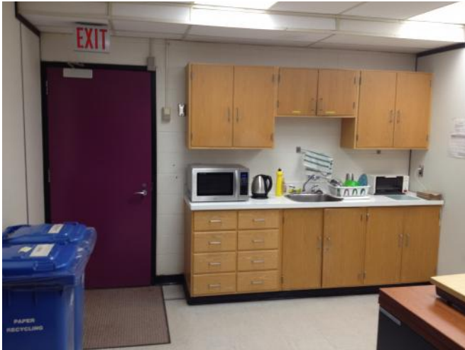
Photograph 5: [2 nd Floor Library] Lead-containing paint applications: purple on walls/doors (Sample ID CCIW-L2), black on walls/door frames (Sample ID CCIW-L3), and white on cinder block walls (Sample ID CCIW-L5).
