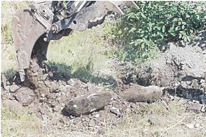
Test Pit #1: Large angular boulder excavated
