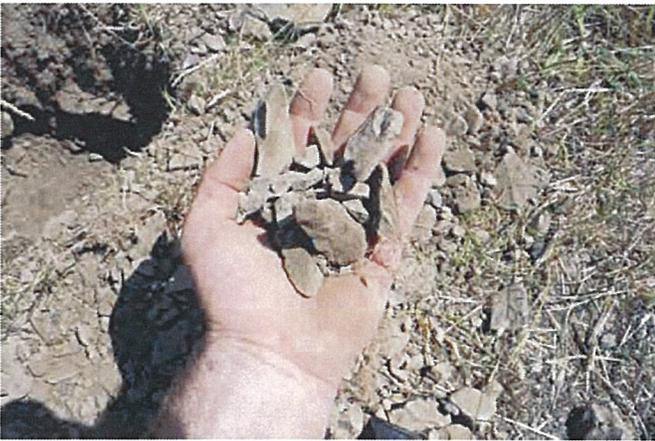
Percolation Hole #1: Sample of coarser material found throughout excavation
