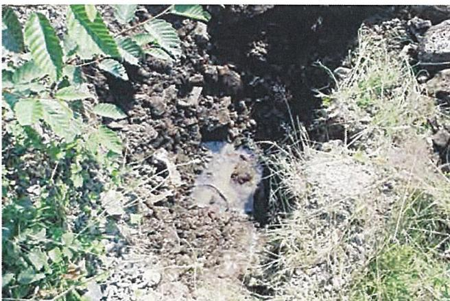
Test Pit #1: Water table observed 1.0m below surface.
