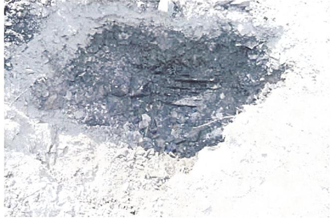
Test Pit #2: Bedrock shale encountered at end of excavation
