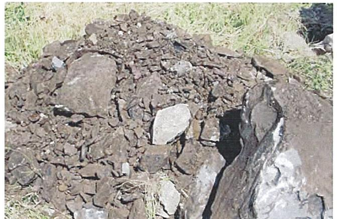
Test Pit #1: Sample of excavated material
