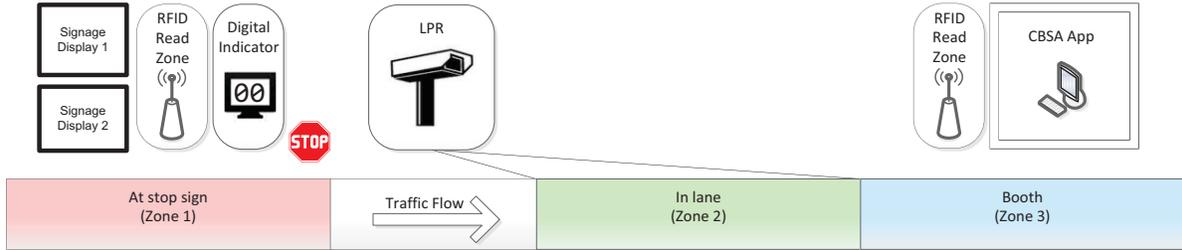
6) 1 RFID read zone in lane + 1 Digital Indicator + 2 Signage Displays
