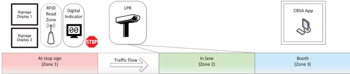
5) LPR + 1 RFID read zone at stop sign + 1 RFID read zone at booth + 1 Digital Indicator + 2 Signage Displays
