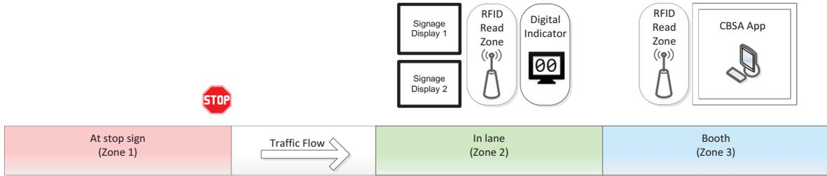
8) 1 RFID read zone at stop sign + 1 Digital Indicator + 2 Signage Displays
