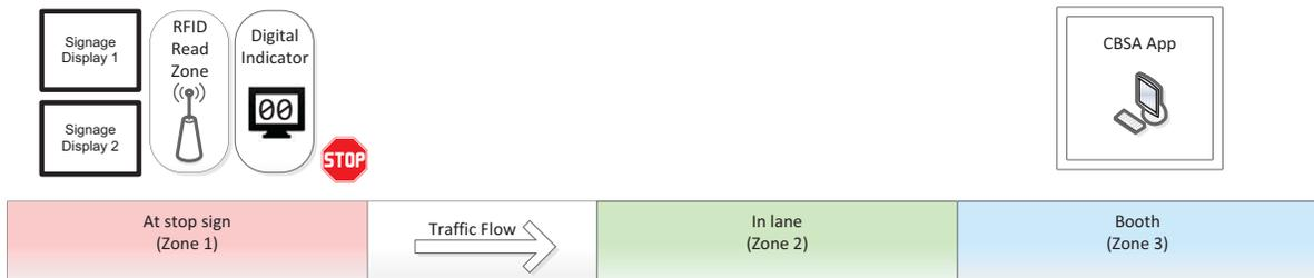
9) 1 RFID read zone at stop sign + 1 RFID read zone at booth + 1 Digital Indicator + 2 Signage Displays
