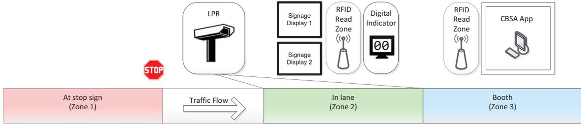
4) LPR + 1 RFID read zone at stop sign + 1 Digital Indicator + 2 Signage Displays
