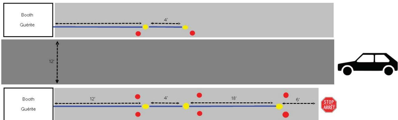
The typical lane is approximately 12ft wide and 40ft long. In front of each Primary Inspection Line (PIL) booth is an asphalt or concrete island that contains two  $\frac{3}{4}$ " or 1" conduits. One conduit contains Category 6 or Category 5e as well as low voltage electrical wires. The other
