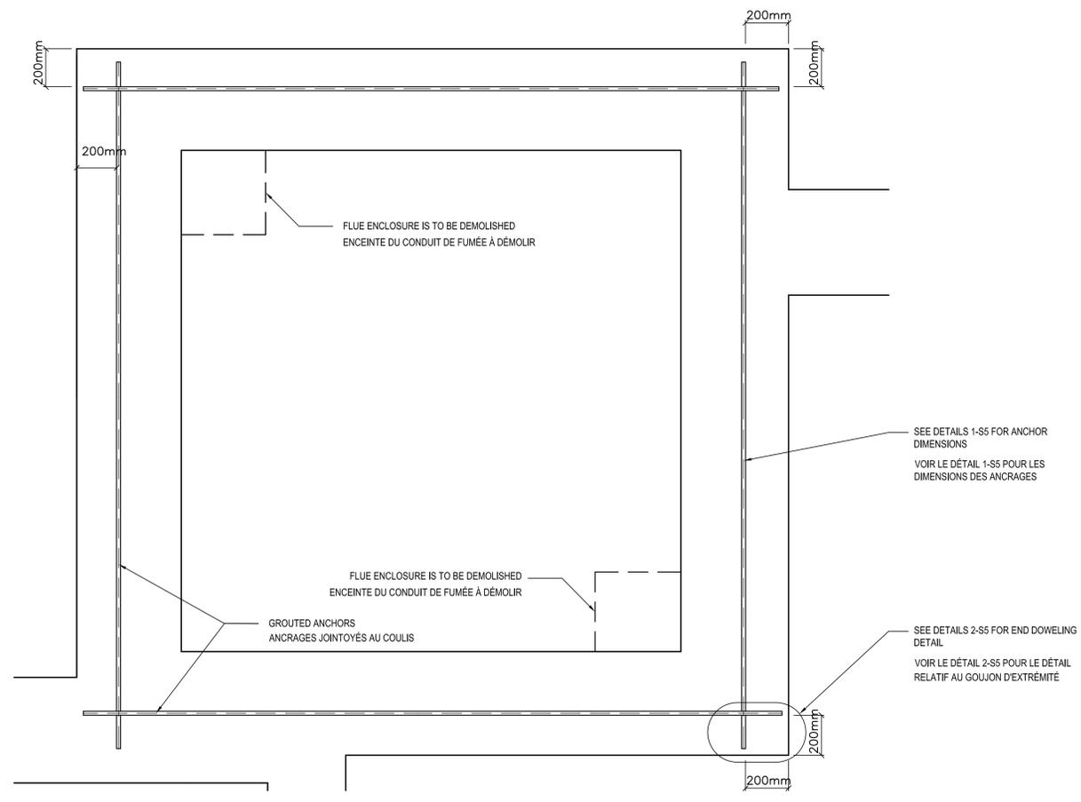
3 HORIZONTAL SECTION IN THE TOWER ILLUSTRATING THE GROUTED ANCHORS
