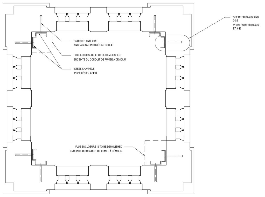
2 HORIZONTAL SECTION AT THE TOP OF THE TOWER ILLUSTRATING THE VERTICAL REINFORCEMENT
