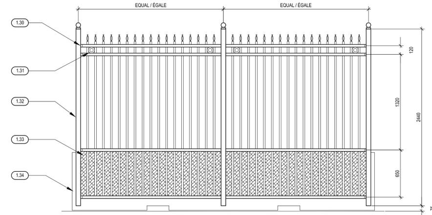
1 FENCE DETAIL (TYP) - ELEVATION
