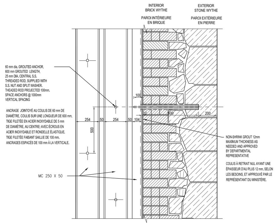
4 VERTICAL SECTION DETAIL AT MC 250 X 50
