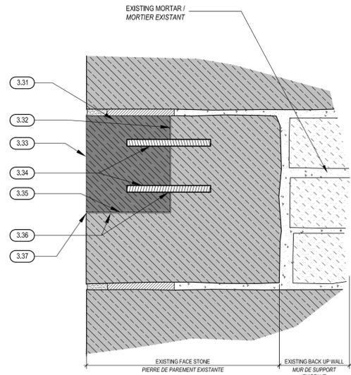
**DUTCHMAN REPAIR:** CUTTING OUT DAMAGED PORTION OF STONE AND PLACING NEW STONE INSERT TO FIT CAVITY. SURFACE OF NEW STONE TO MATCH ADJACENT EXTERIOR SURFACE. / **RÉPARATION PAR MORCEAU RAPPORTÉ:** DÉCOUPER LA PARTIE ENDOMMAGÉE DE LA PIERRE ET REMPLACER PAR UNE NOUVELLE PIERRE QUI S'AJUSTE BIEN DANS LA CAVITÉ. LA SURFACE DE LA NOUVELLE PIERRE DOIT ÊTRE ASSORTIE À LA SURFACE EXTÉRIEURE ADJACENTE.
