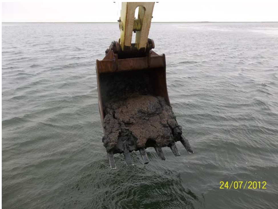
Photo 5 - Dark silt with organics encountered at TP 1 - McEachern's Point (Elev. -1.60 to -2.60 CD).
