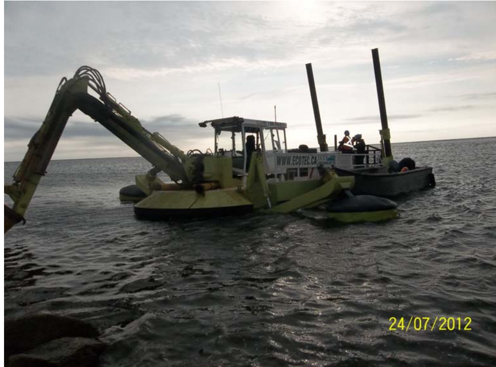
Photo 2 - Amphibian excavator in McEachern's point channel.
