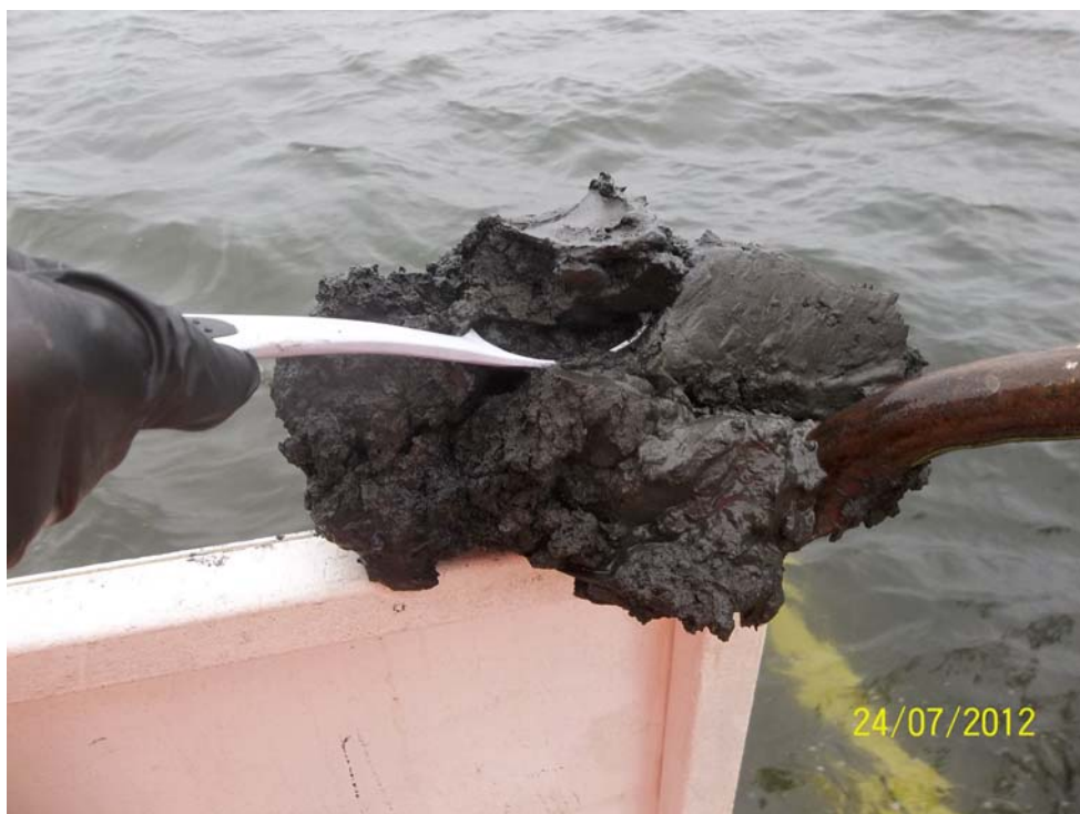
Photo 6 - Dark grey silt encountered at TP 2 - MaEachern's Point (Elevation -1.34 to -2.34 CD).
