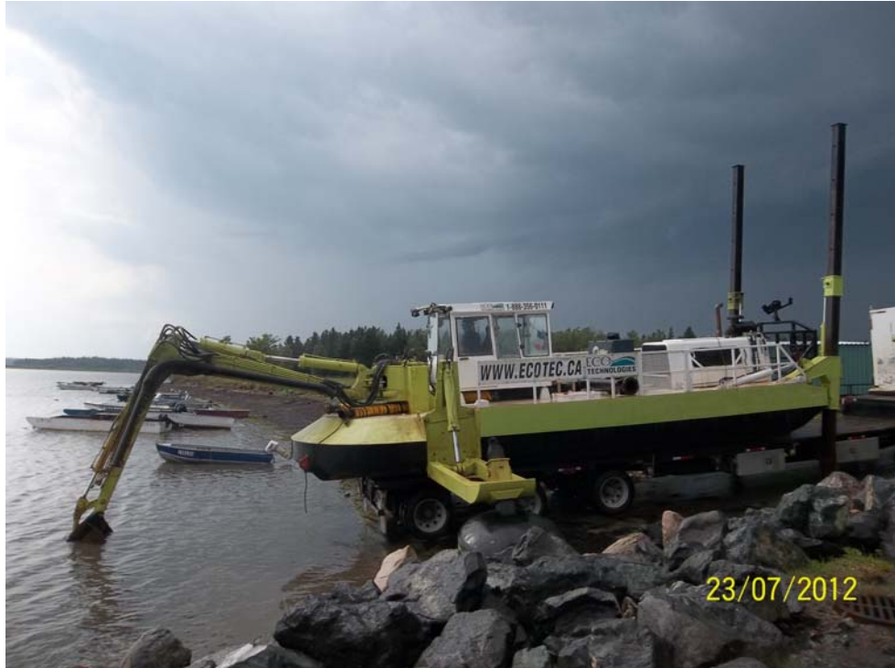
Photo 1 - ECO Technologies Aphibian Excavator at McEachern's Point Wharf.
