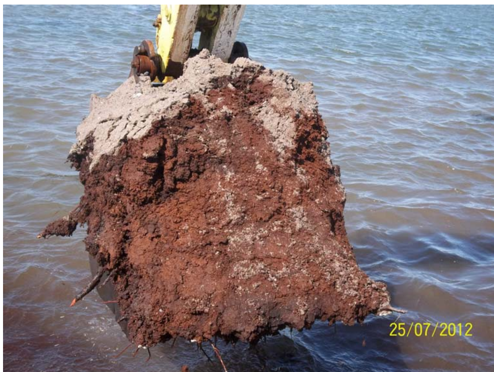
Photo 14 - Thick peat layer encountered at TP 10 - MaEachern's Point (Elevation – 0.47 to –1.12 CD).
