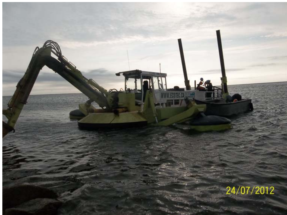
Photo 2 - Amphibian excavator in McEachern's point channel.
