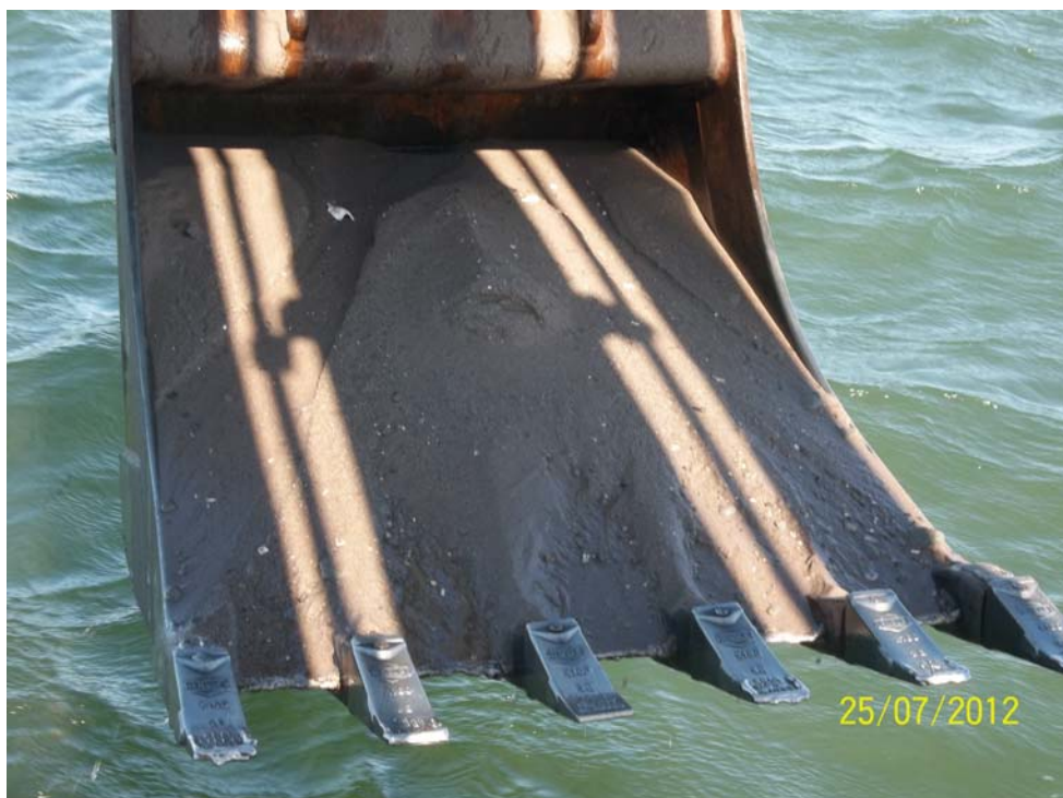
Photo 16 - Brown sand with some cobbles and organics encountered at TP 12 - McEachern's Point (Elevation -1.03 to -1.53 CD).
