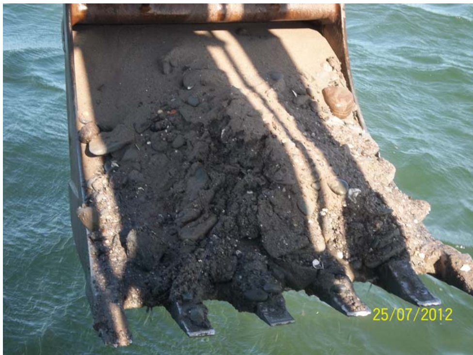
Photo 17 - Brown sand and gravel with cobbles and organics encountered at TP 13 - McEacherns Point (Elevation -1.22 to -1.72 CD).
