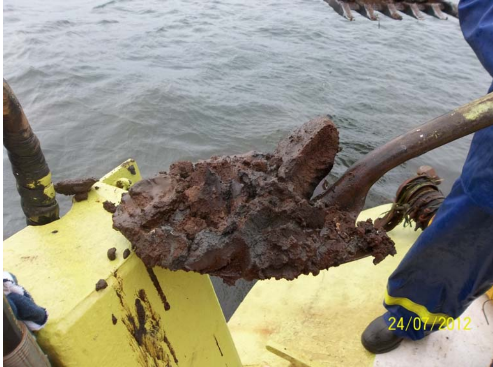
Photo 11 - Brown silty sand with trace gravel and wood debris encountered at TP 7 - McEachern's Point (Elevation -1.00 to -1.85 CD).
