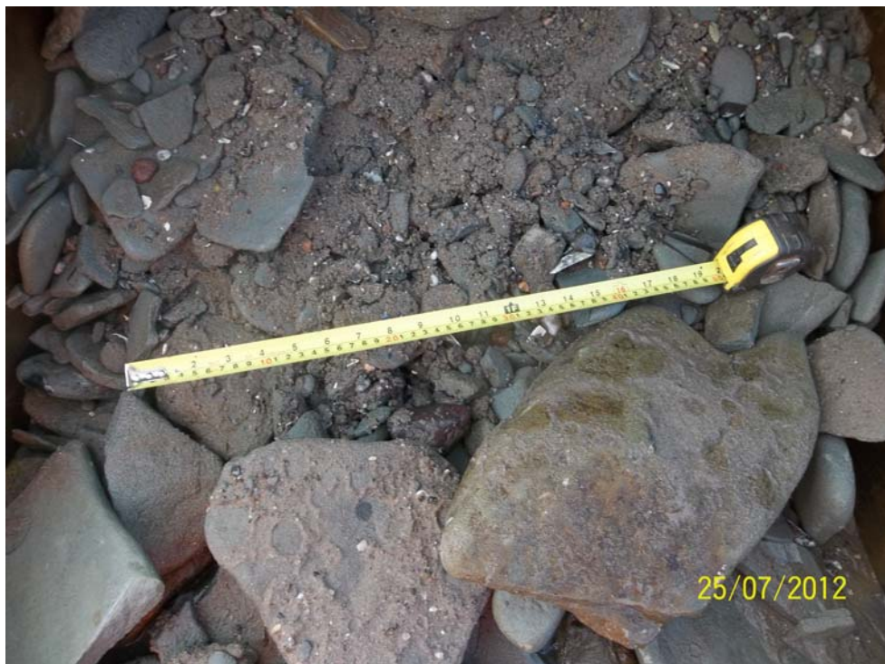
Photo 19 - Brown sand and gravel with cobbles and boulders encountered at TP 15 - McEachern's Point (Elevation -1.40 to -2.90 CD).
