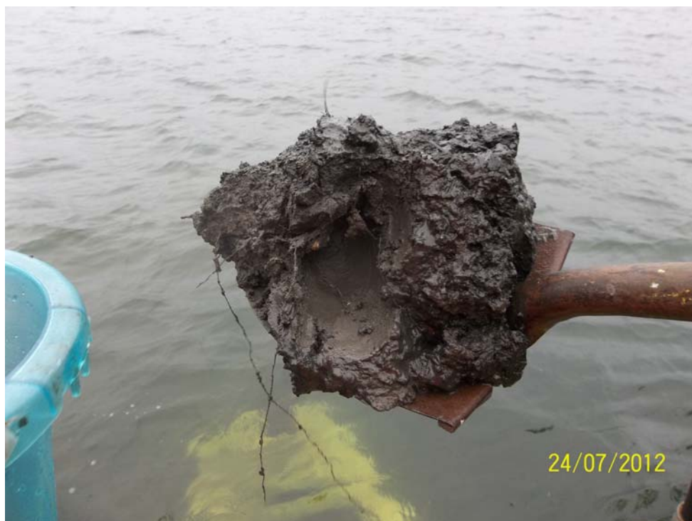
Photo 9 - Dark grey silt with some organics at TP 5 - McEachern's Point (Elevation – 1.29 to –2.49 CD).
