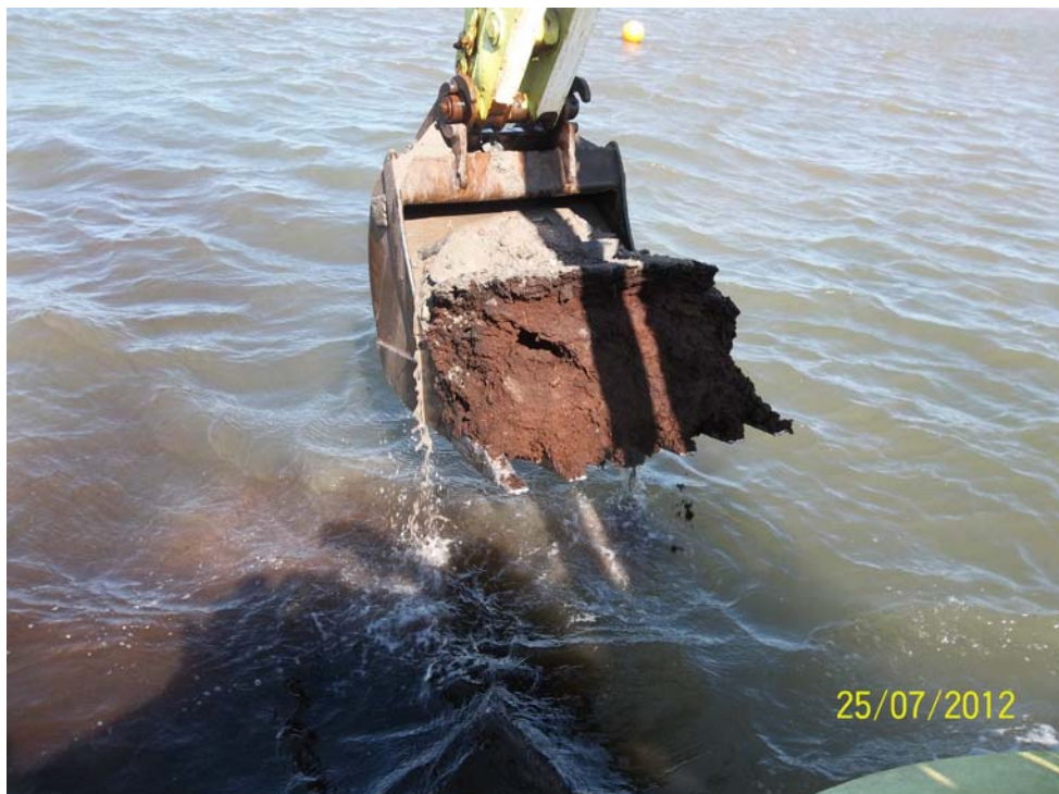
Photo 15 - Thick layer of peat encountered at TP 11 - McEachern's Point (Elevation -0.60 to -1.15 CD).
