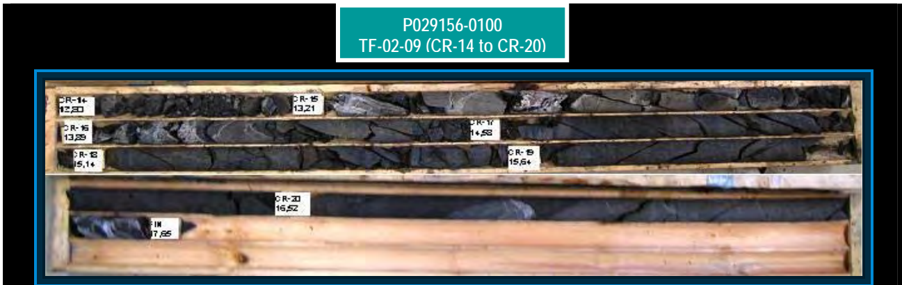
PHOTO #20: Rock core samples (CR-14 to CR-20) taken from the TF-02-09 borehole, from a depth between 12.80 and 17.65 metres below the seabed.
