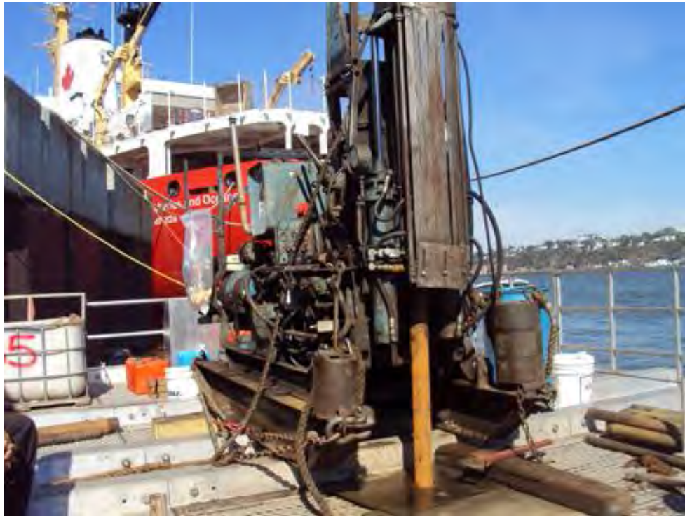
Photo 3 : Foreuse BBS 18 installée sur la barge / BBS-18 drill installed on a floating barge
