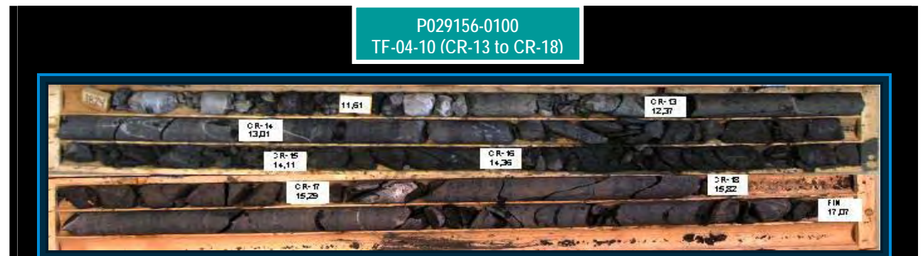
PHOTO #22: Rock core samples (CR-13 to CR-18) taken from the TF-04-09 borehole, from a depth between 12.37 and 17.07 metres below the seabed.
