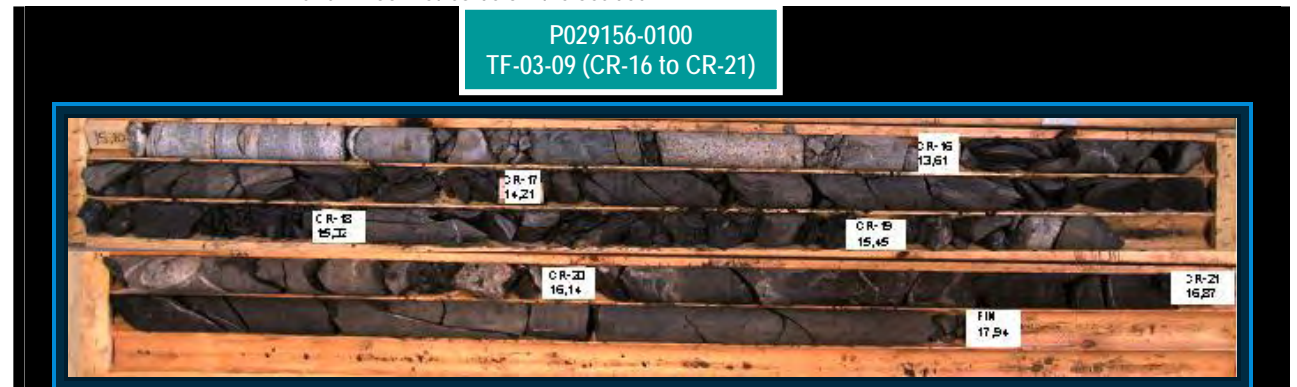
PHOTO #21: Rock core samples (CR-16 to CR-21) taken from the TF-03-09 borehole, from a depth between 13.61 and 17.94 metres below the seabed.
