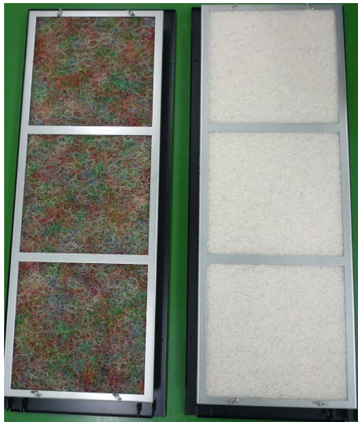
(Right: for Air Intake, Left: for Exhaust Ventilation)
