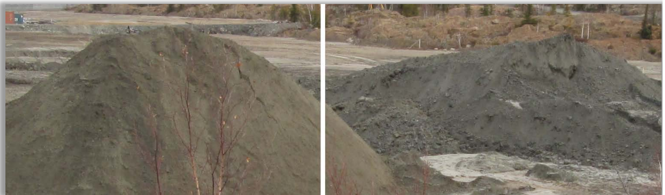
Figure 1: Comparison of prepared tailings stockpiles - left: Stockpile #2 used during paste trial; right: Stockpile #1 unusable for paste trial.
