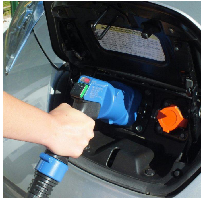
Figure 16. CHAdeMO connector seated in vehicle
