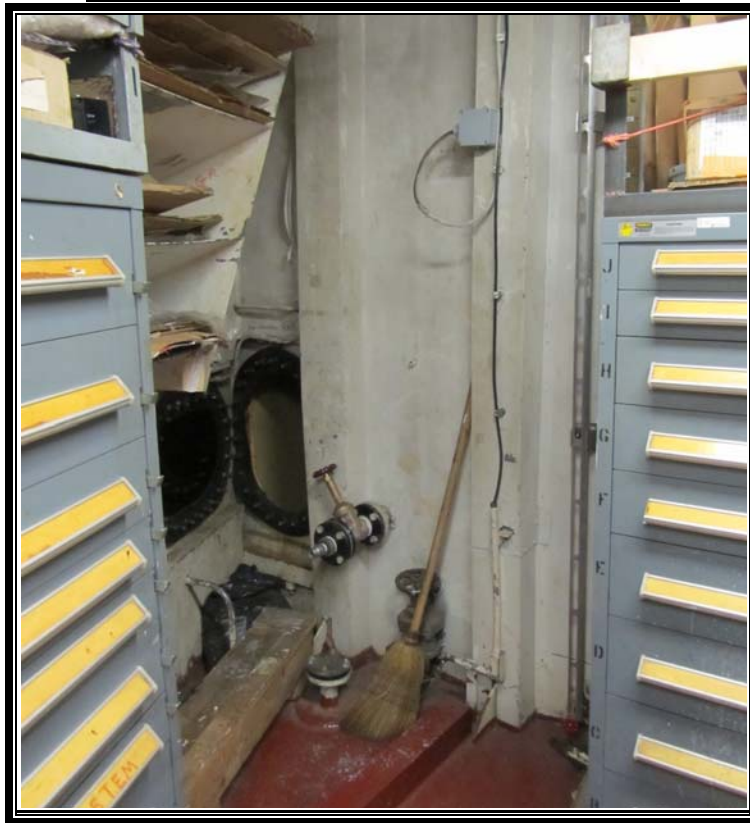
Access to tank from Manhole on Aft Bulkhead
