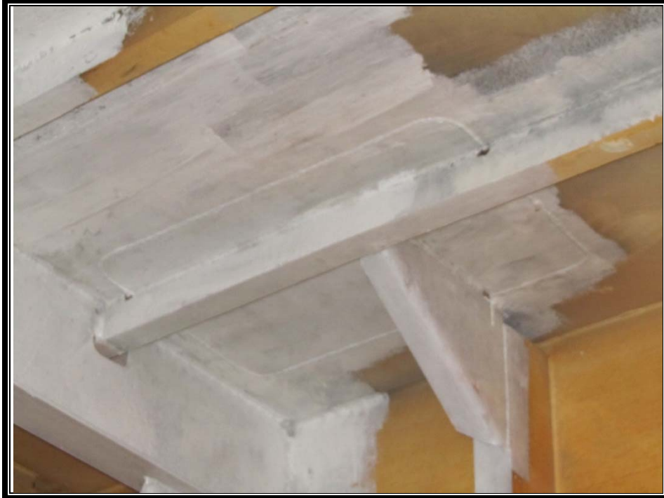
Tank Top - Section of Plating & Transverse Deep Beam Renewed( See attached Dwg.)
