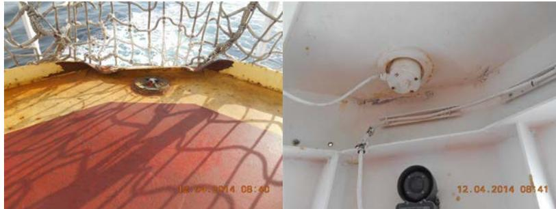
3.4 All new and disturbed metal shall receive two coats of primer and one topcoat of Amercoat 5450.
