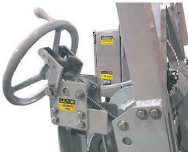
Figure 21: Locking Handle - Stowed Position
