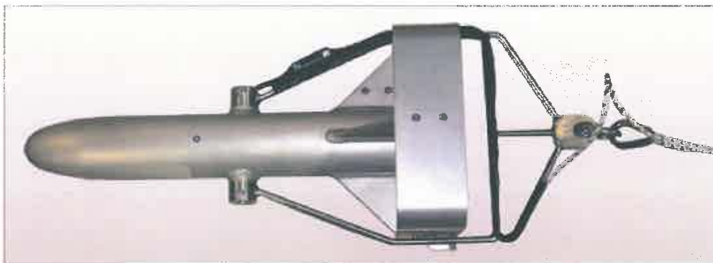
Figure 24: Tow Cable Installed on Bridle
