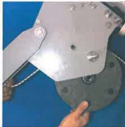
Figure 19: Inserting the Tow cable in A-Frame Sheave
