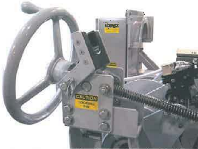
Figure 20: Locking Handle - Overboarding Position
