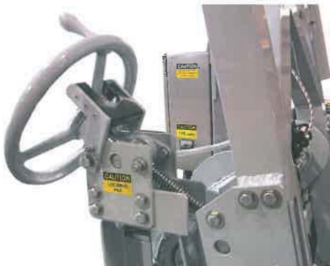
Figure 21: Locking Handle - Stowed Position
