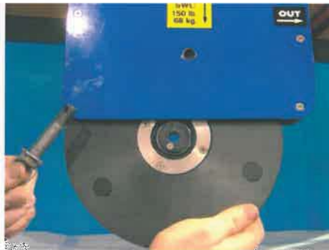
Figure 15: Removing Sheave Axle Bolt
