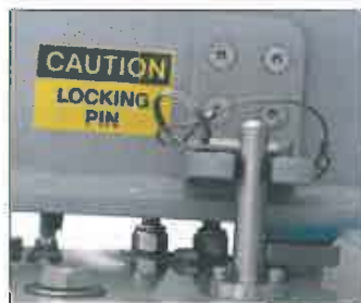
Figure 8: A-Frame Sheave Locking Pin
