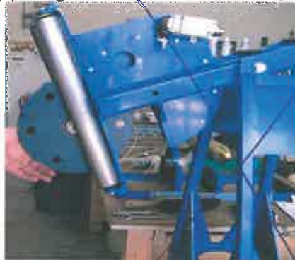
Figure 12: Removing the Sheave
