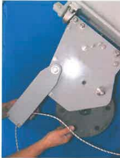
Figure 18: Removing the Sheave
