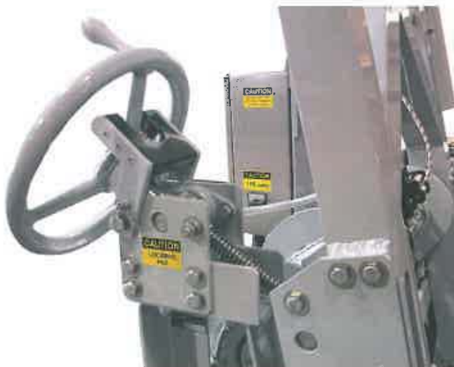
Figure 21: Locking Handle - Stowed Position
