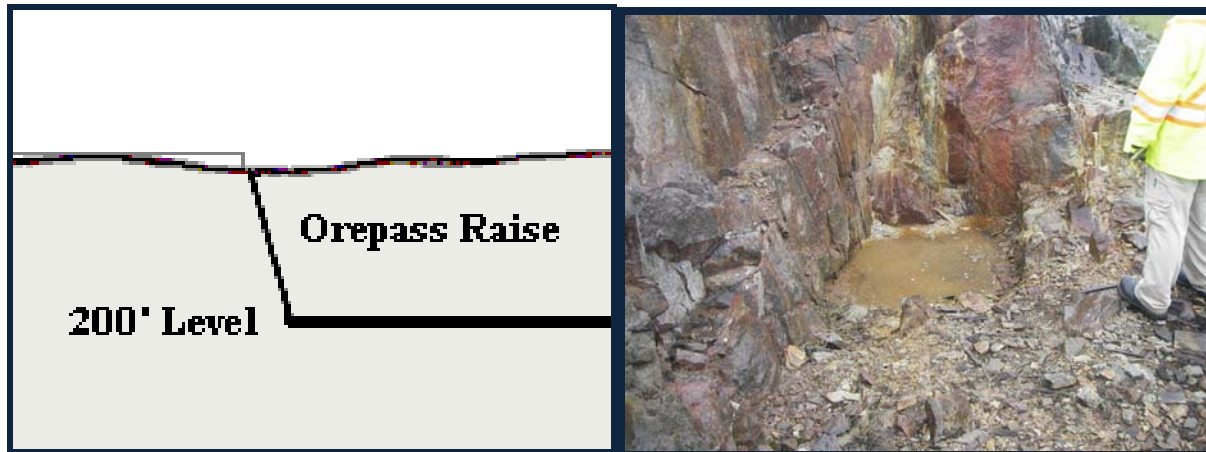
Figure 3. Section through Orepass Raise (left); photo of concrete cap (right).
