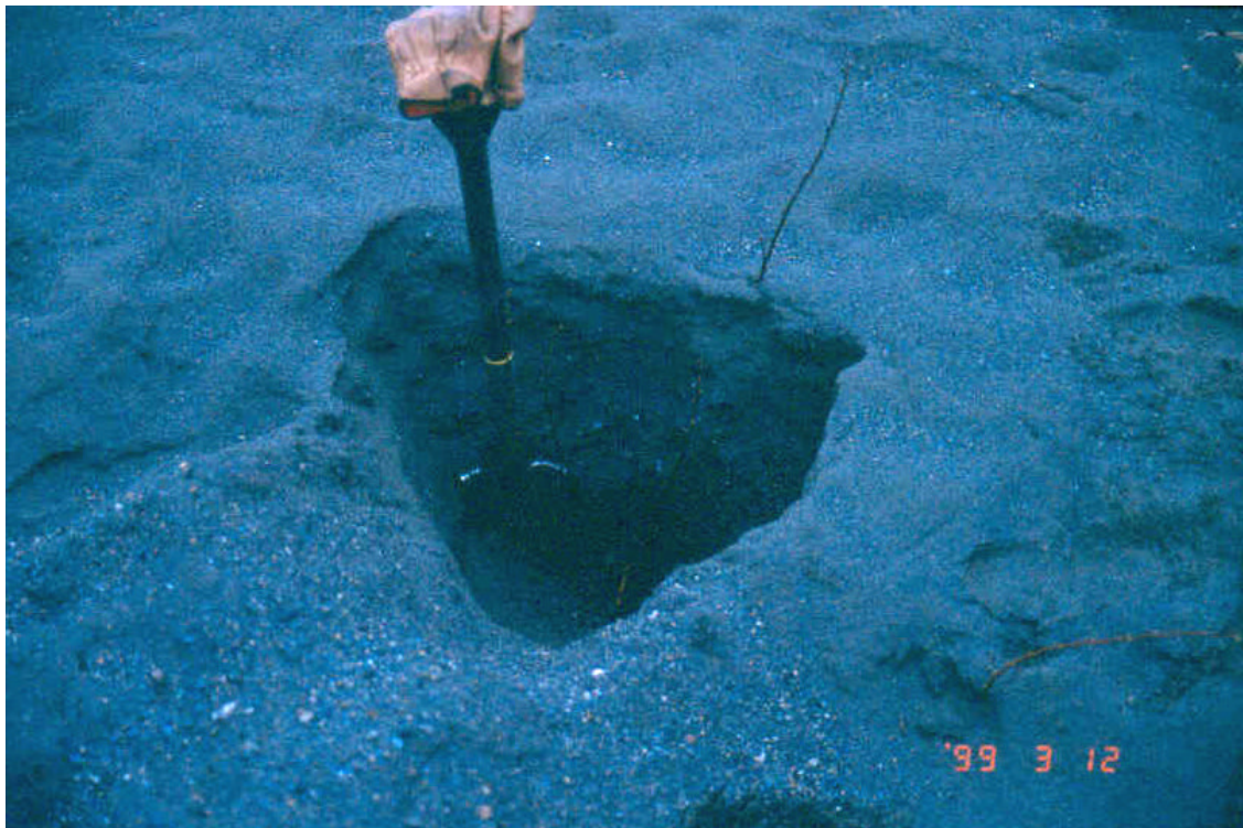
Photograph 5.3.4-1. Over 80 cm of sediment was deposited on this gravel bar on the San Juan River following live gravel bar staking (from Polster, 2001).
