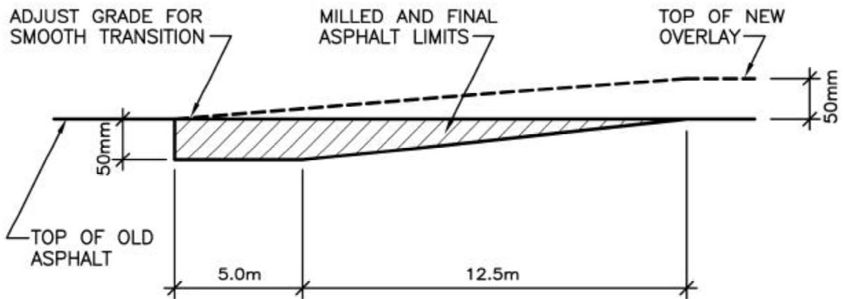
TIE FROM EXISTING TO NEW ASPHALT OVERLAY
