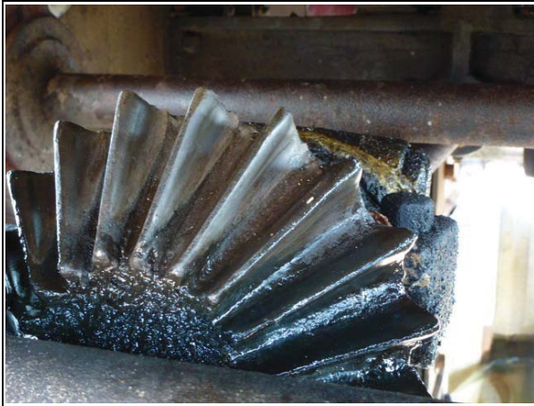
Figure 6 - Gear R3L (mate to Gear R4L). Gear R3R is identical, but located at opposite end of stoplog lifting machine.
