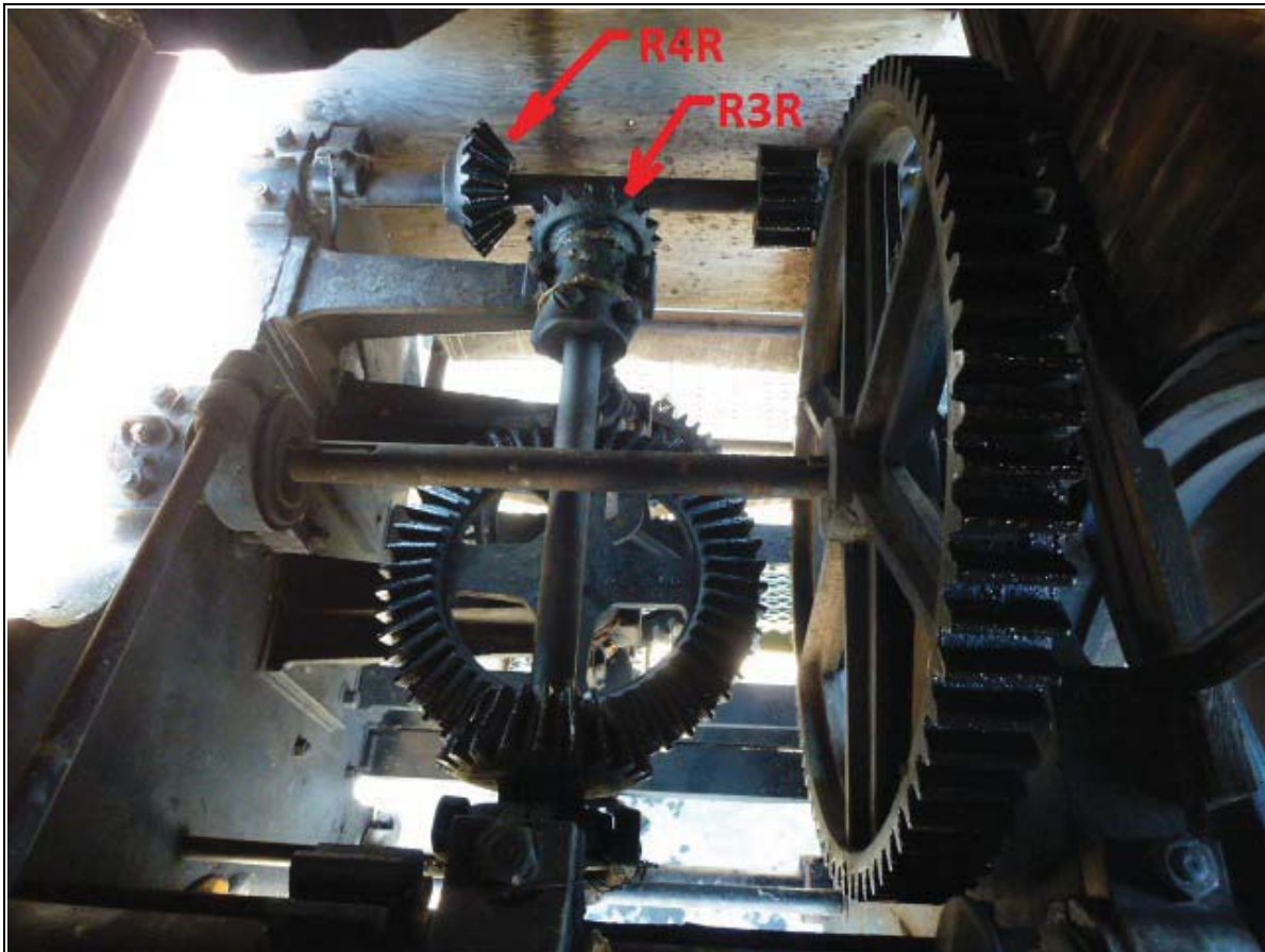
Figure 8 - Gear train at right end of stoplog lifting machine, showing R3R/R4R pair (not engaged in this photo). The gear pair R3L/R4L are mirror-image at the other end of the stoplog lifting machine.
