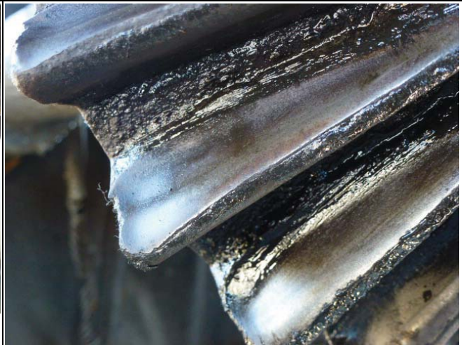
Figure 7 – Detail of Gear R4L (mate to Gear R3L). Gear R4R is identical, but located at opposite end of stoplog lifting machine.
