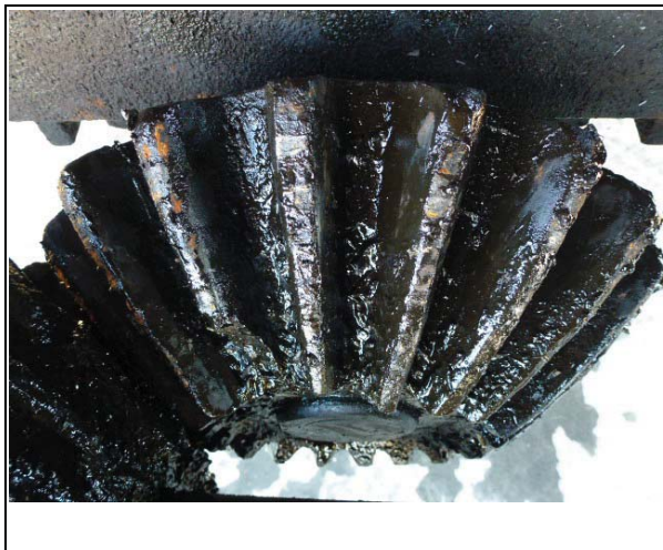
Figure 4 - Gear T9L (mate to Gear T10L, of which a few teeth are visible at lower left of photo).
