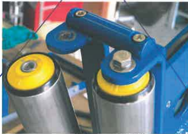
Figure 10: Loosened Roller
