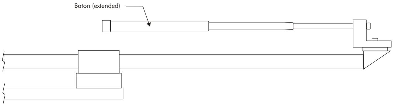
Position of Pneumatic Cylinder Driven Ram at end of opening action (baton extended)
