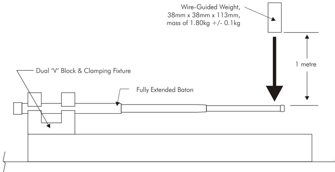
Side Strike Test Apparatus
