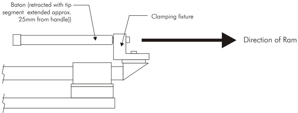
Position of Pneumatic Cylinder Driven Ram at start of opening action (baton retracted)
