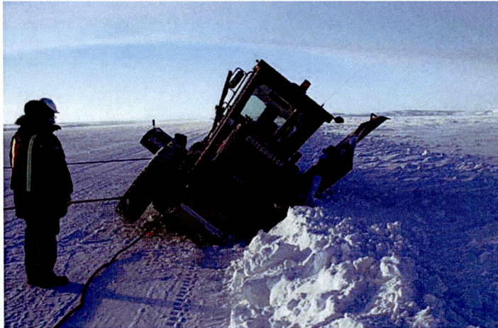
Figure 25 Grader partially broken through thin ice beneath a snowbank
