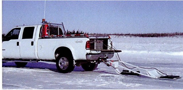
Figure B1 Dual channel GPR ice profiling equipment (being pulled behind a truck) measuring ice thickness and water depth in a single pass
