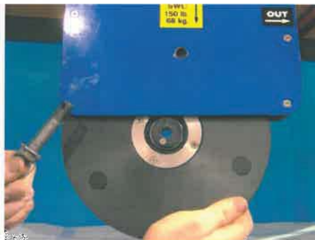
Figure 15: Removing Sheave Axle Bolt
