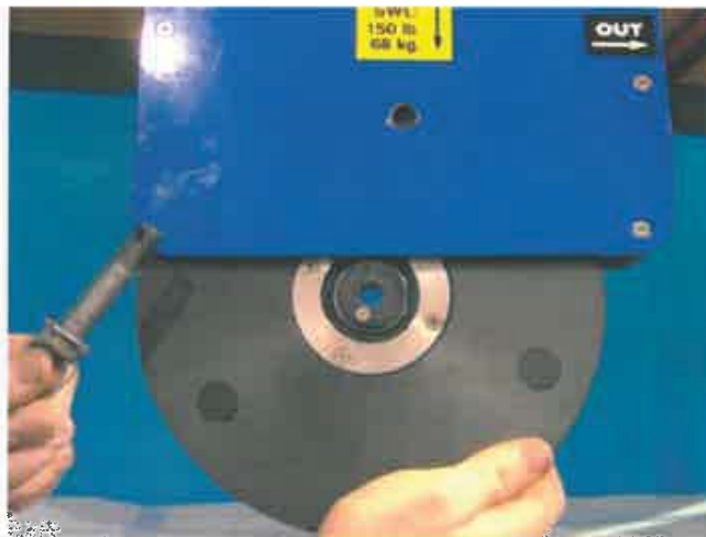
Figure 15: Removing Sheave Axle Bolt
