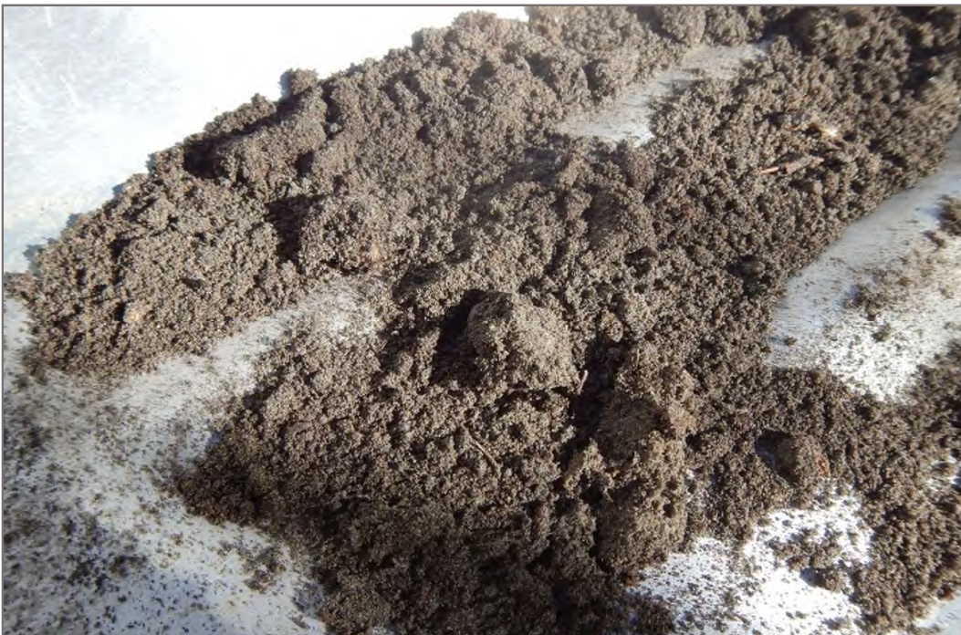
Photo 14: SAND, silty, surface organics, brown to grey, damp; fine sand. Large trees present on portions of this slope, up to 30 cm diameter. Photo Taken March 4, 2014
