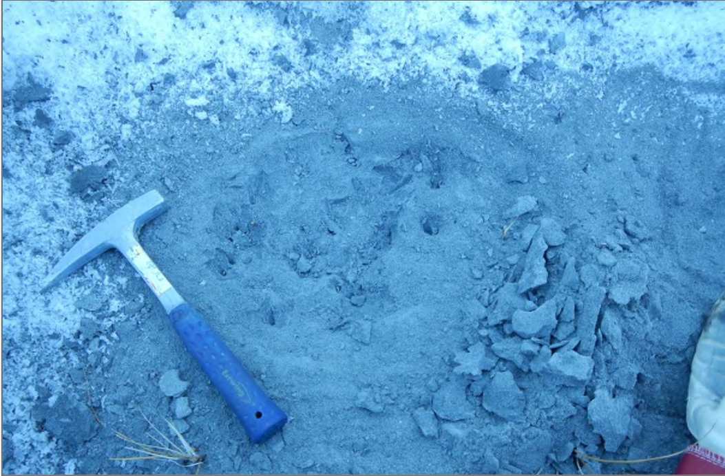
Photo 3: South bank beach underneath ferryway cable. Soil is fine SAND, with some silt, dry near the surface and frozen/hard just below. Photo Taken March 4, 2014
