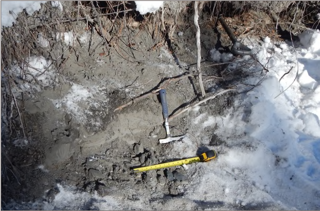
Photo 5: Closeup of scour zone on the north bank. By the hammer head, the soil becomes rounded gravel and sand. The fragments are frozen chunks of sand. Photo Taken March 4, 2014
