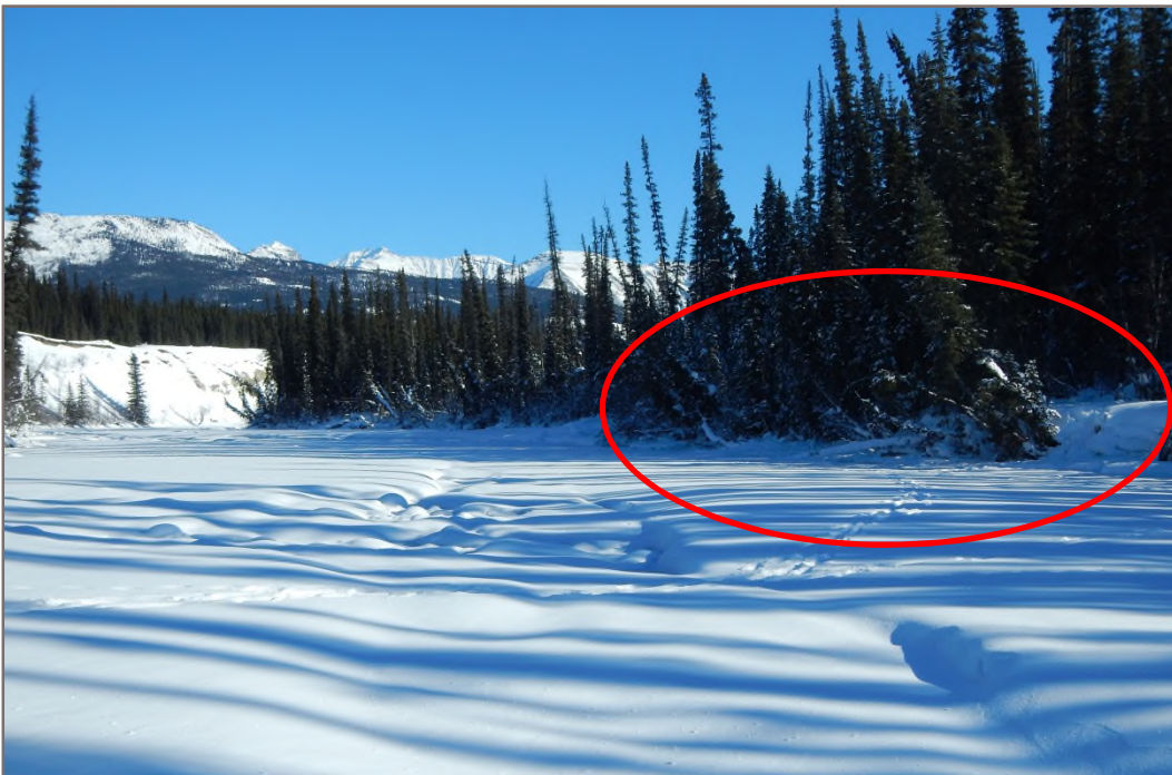
Photo 10: View looking east downstream at area mapped as colluvial terrace on south bank. The trees on the right side of the photo are just upriver of the ferryway structure where the hillside appears to be gradually slumping or subsiding into the river. Photo Taken from Helicopter landing site, March 4, 2014
