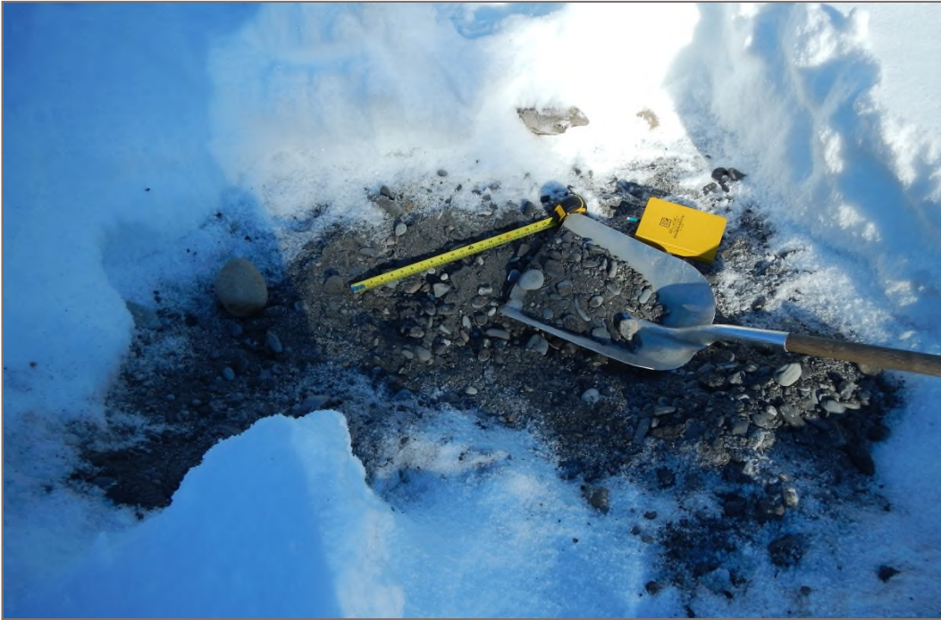
Photo 1: North bank gravel bar, upriver of ferryway structure. Aggregates up to 125 mm in diameter. Photo Taken March 4, 2014
