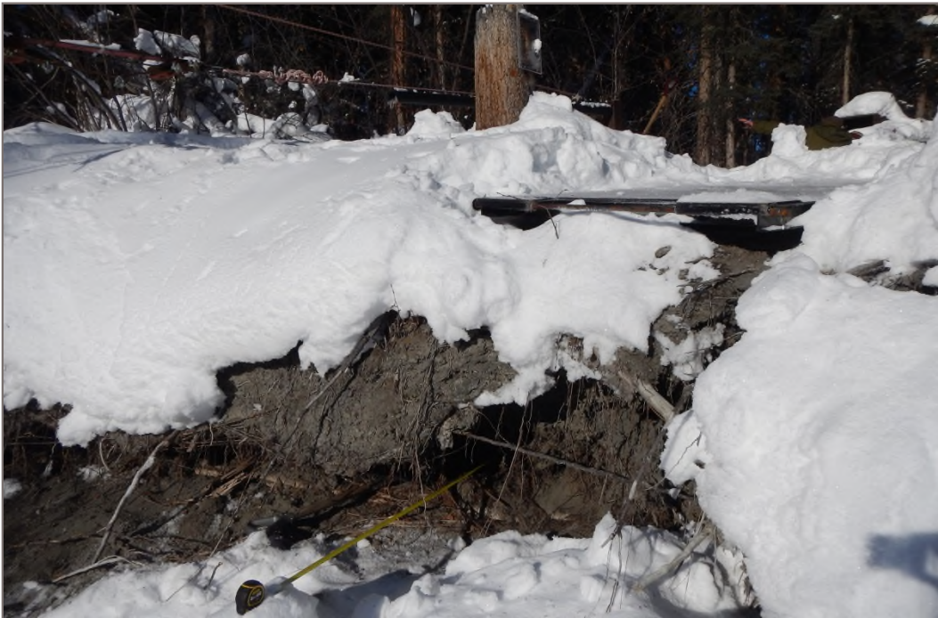
Photo 4: North bank erosion underneath ferryway cable. Test drilling within the scour zone showed sandy soils and a gravel interbed. The scour has resulted in a 0.9 overhang. Photo Taken March 4, 2014
