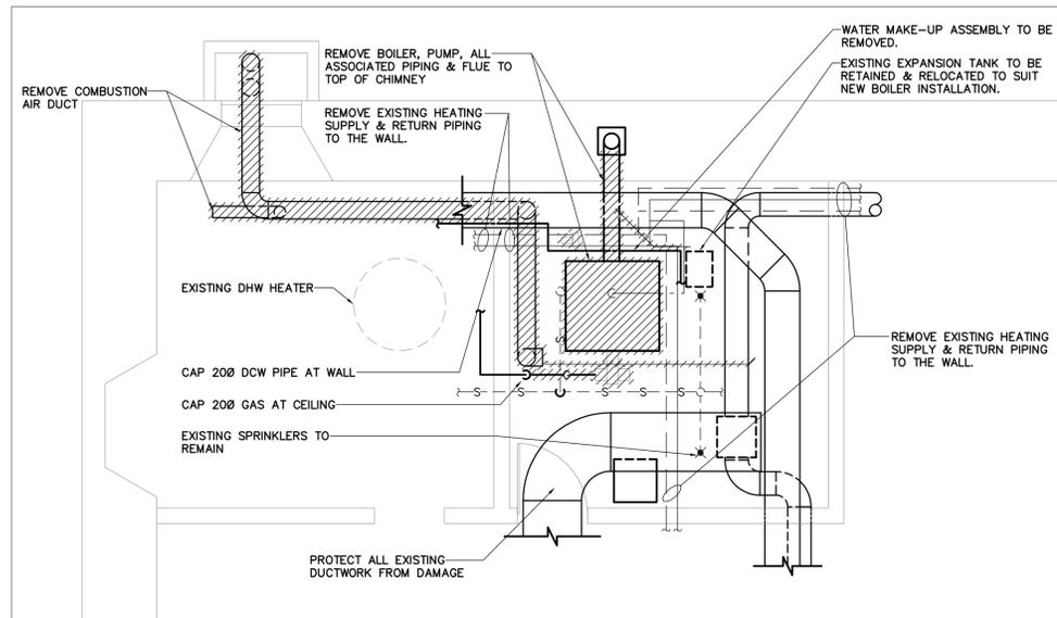
**1 PART BASEMENT FLOOR PLAN DEMOLITION - MECHANICAL**
