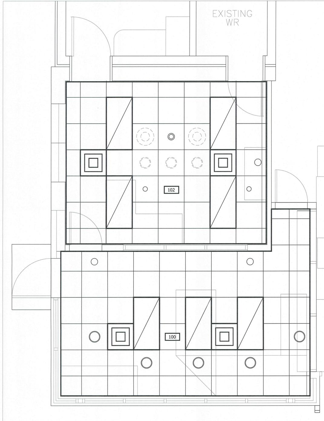
NEW ACOUSTICAL TILES TO BE PROVIDED & INSTALLED IN ROOMS 100 & 102 (610 x 1220)
