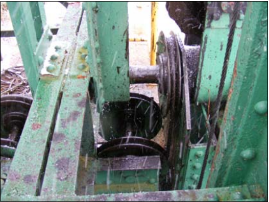
39 H16 PULLEYS AND CABLES (GATE LIFTING MACHINERY)
