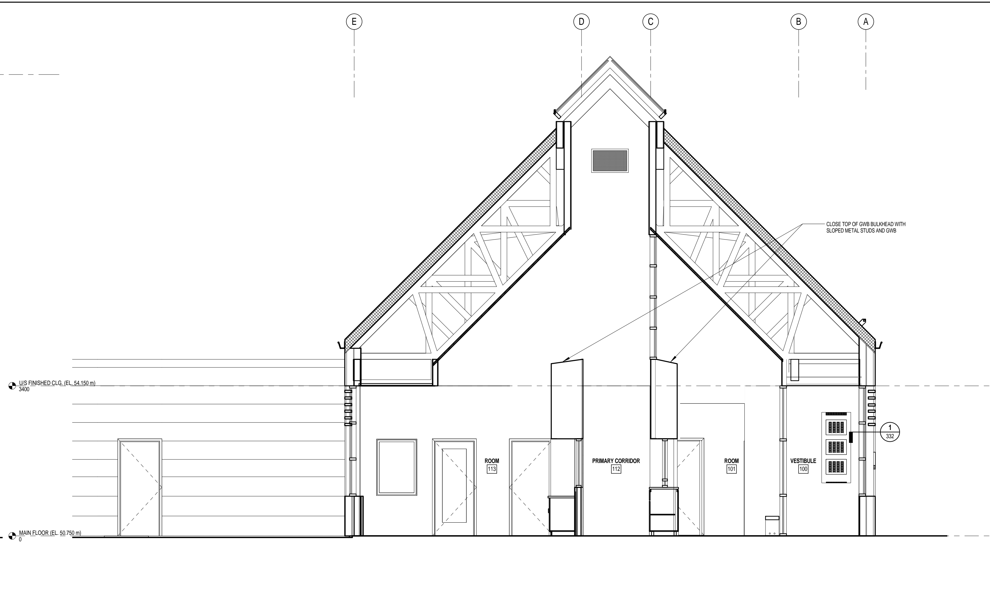
2 SECTION THRU ENTRY VESTIBULE AND RECEPTION 301 1:50
