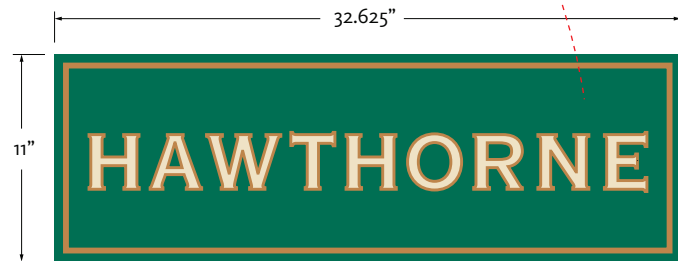
Street Name Decal (screen printed vinyl, scale 1:10)
