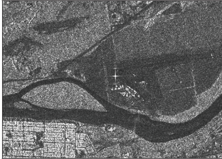
Figure 1 Response of a transponder installed on the Prince Albert (SK) airport grounds, visible in a RADARSAT-1 scene.
