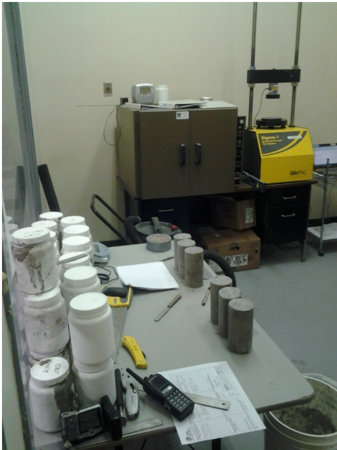
Figure 2: UCS Lab Equipment as set up at Giant Mine M.E.G. Facility.
