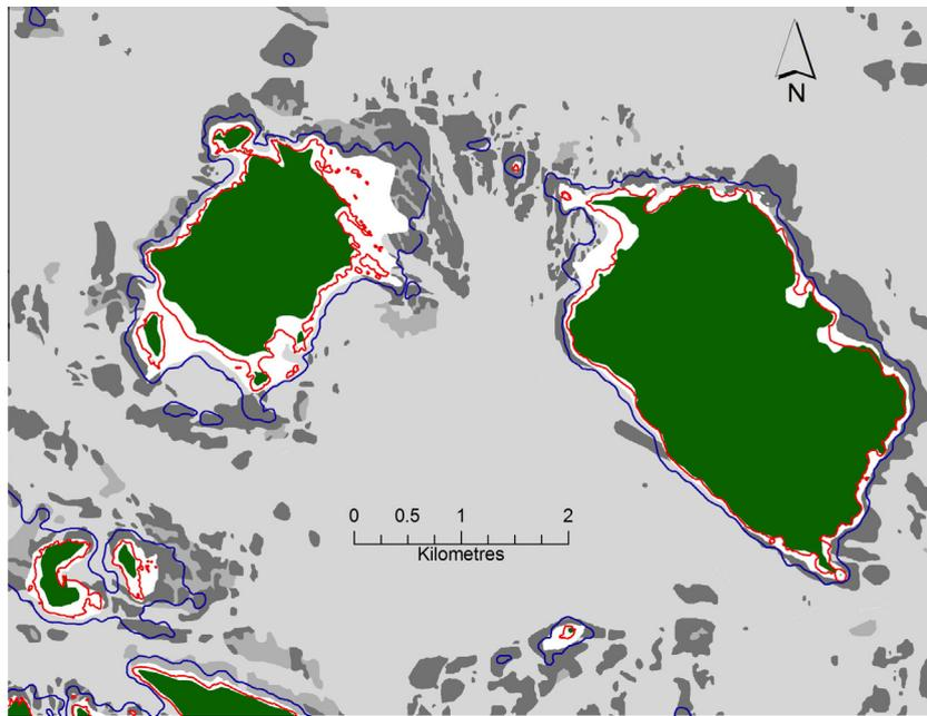
**Fig. 1.** Illustration of the extents of the 'white strip' around islands in the Strait of Georgia. Contour lines (red = low water line; blue = 10 m) are shown over top of bottom type classes (grey scale, hard is dark, soft is light) derived from morphological analysis that included acoustic multibeam backscatter data (Greene and Barrie, 2011). (For interpretation of the references to colour in this figure legend, the reader is referred to the web version of this article.)
