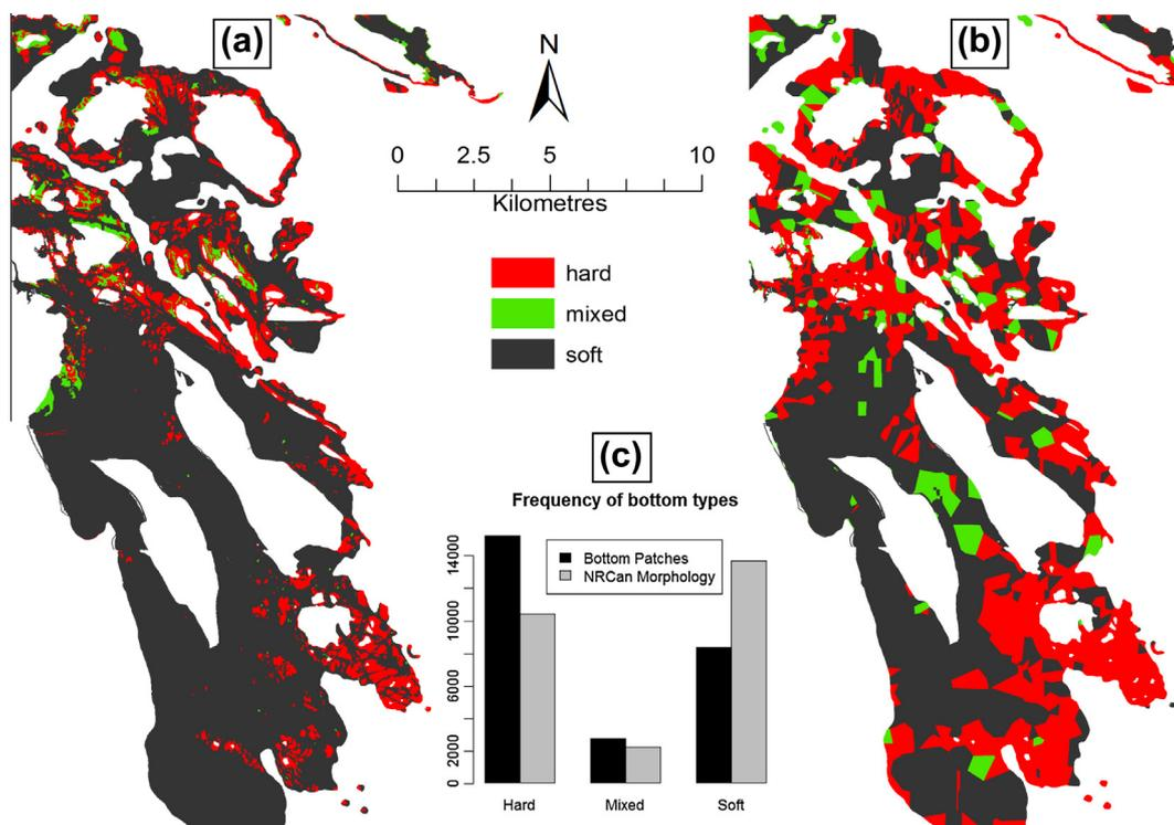
**Fig. 8.** Hard, mixed, and soft bottom types according to (a) a traditional morphological analysis based on bathymetry, rugosity, and multibeam backscatter information (from Greene and Barrie, 2011), and (b) the bottom patches derived herein for a portion of the study area. The frequency of the different bottom types (c) shows that the bottom patches tend to be biased towards hard assignment, possibly at the expense of soft bottom types.
