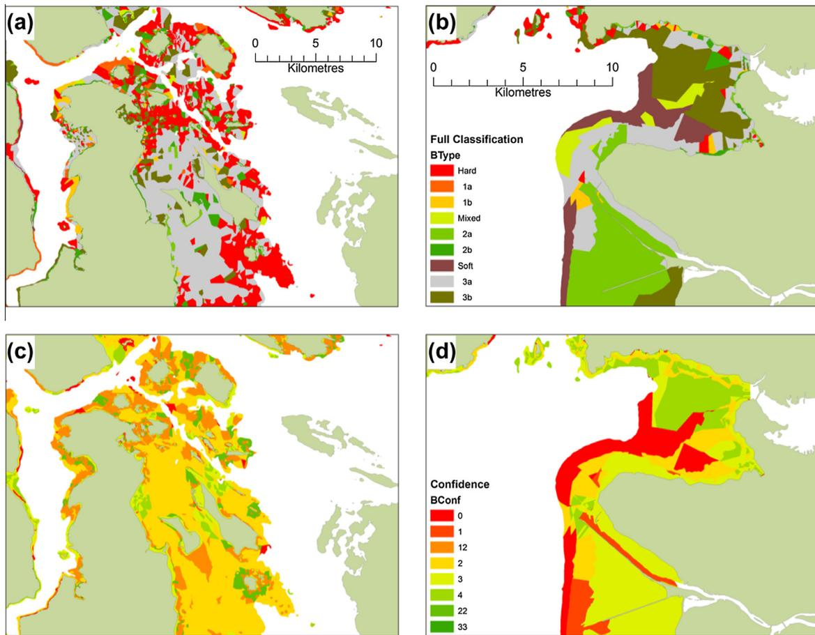
**Fig. 5.** Example of Bottom Patch Classification (BType –a, b) and confidence (BConf –c, d; low = red; high = green) for two representative areas with high (a, c) and low (b, d) expected heterogeneity.
