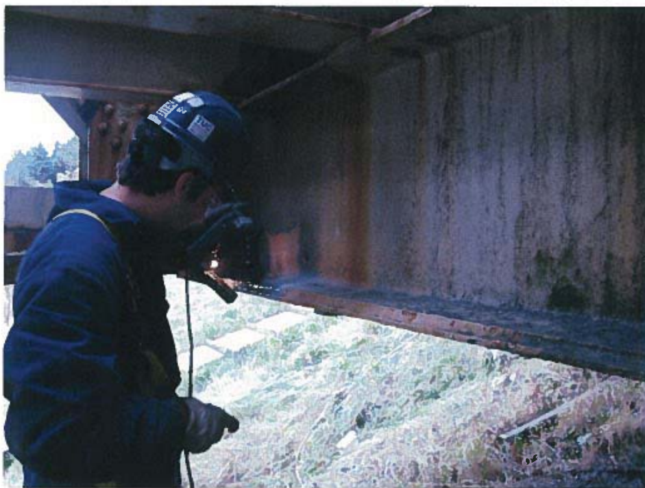
Photograph 45 – Magnetic particle testing of welded reinforcement at bottom flange of floor beam at panel point 2W
