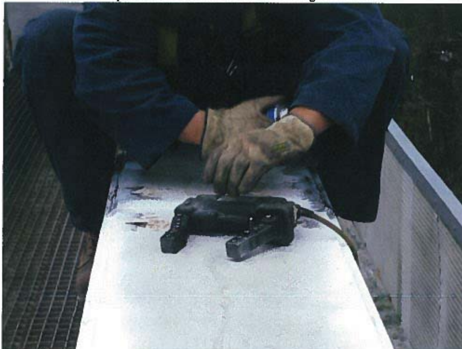
Photograph 40 – Magnetic particle testing of welded reinforcement at south truss top chord between panel points 1E and 3E
