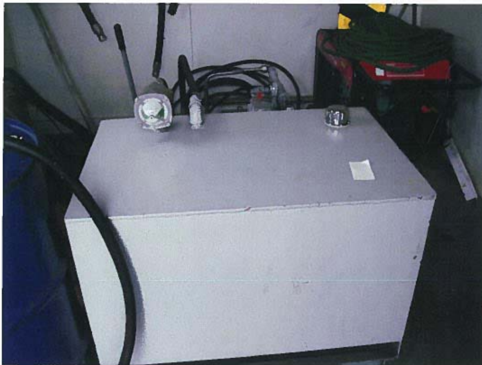
Photograph 10 – Hydraulic power unit 2
