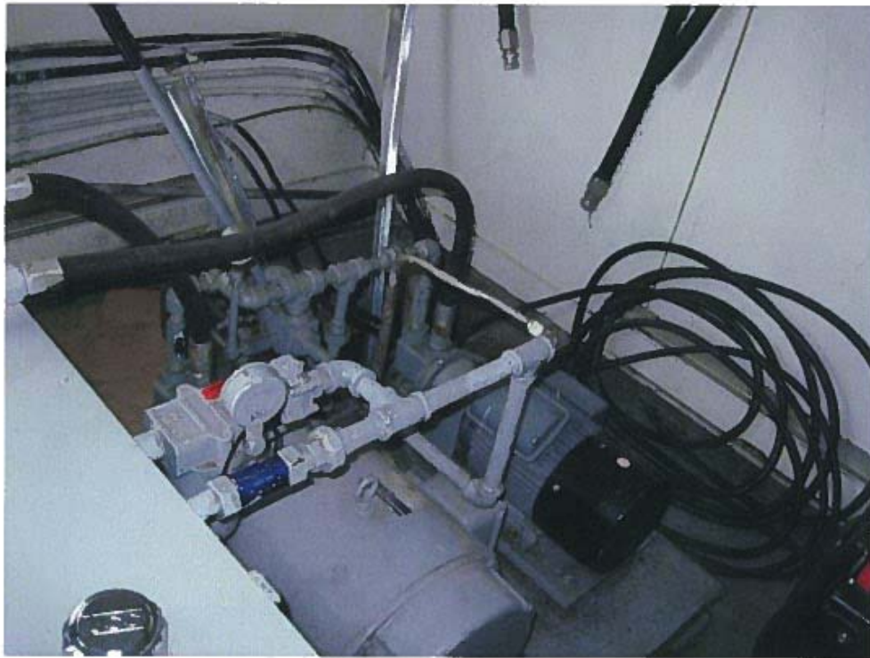
Photograph 9 – Hydraulic power unit 1
