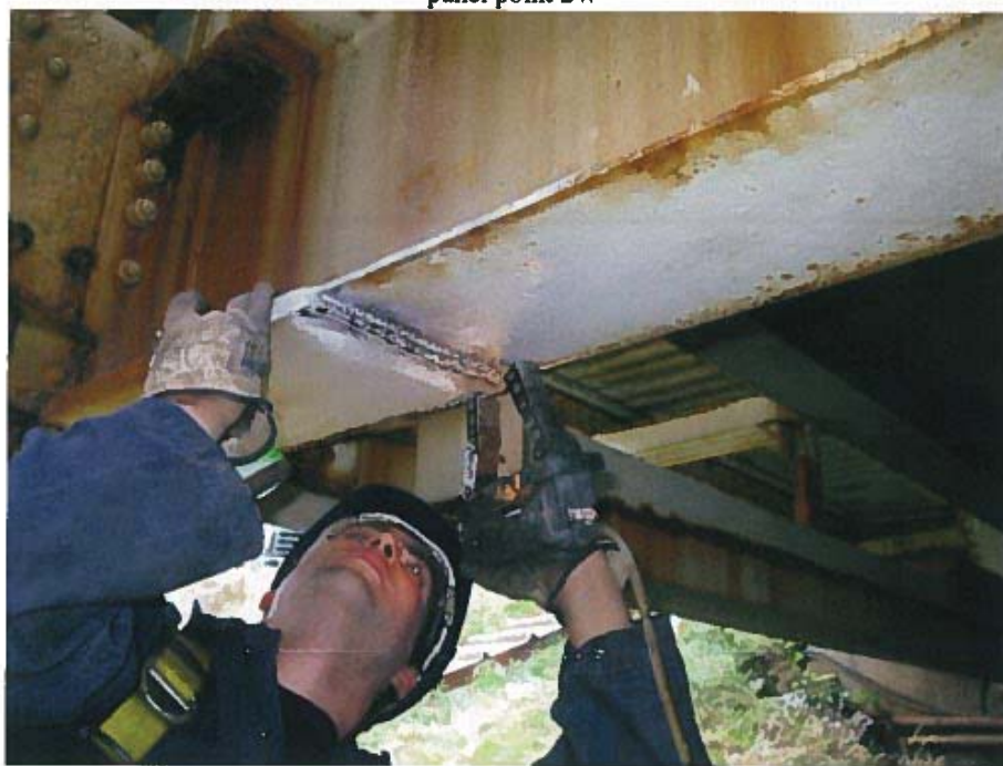
Photograph 46 – Magnetic particle testing of welded reinforcement at bottom flange of floor beam at panel point 2W
