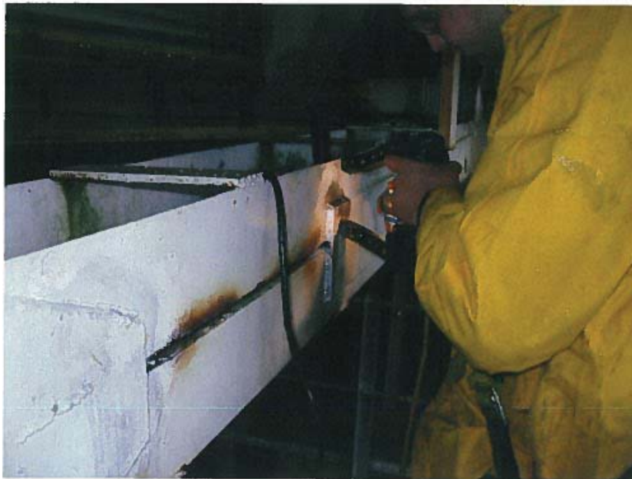
Photograph 50 – Magnetic particle testing of welded reinforcement at south truss bottom chord between panel points 4E and 5E.
