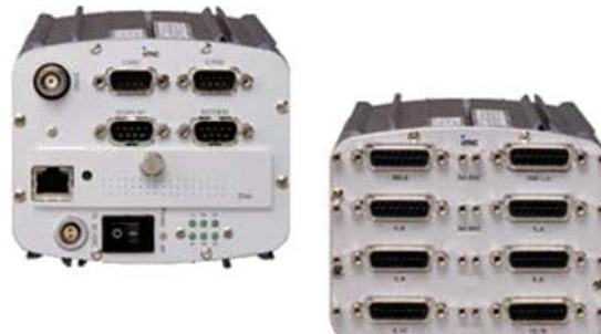
Figure 1 - Front and Back images of the IMC CS-7008 DAQ
