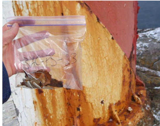
Photo 20: View of paint sample BAC-PS-23.
