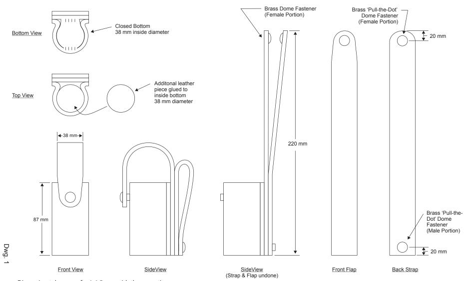
Dimension tolerance of  $\pm$ 1.5 mm with the exception of the inside diameter, which shall have a  $\pm$ 1.5 mm tolerance NOT TO SCALE
