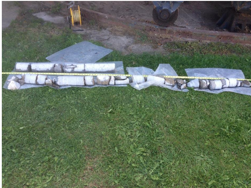
Photograph 2: Corehole CH 13-1 Concrete Cores and full depth Rock Cores
