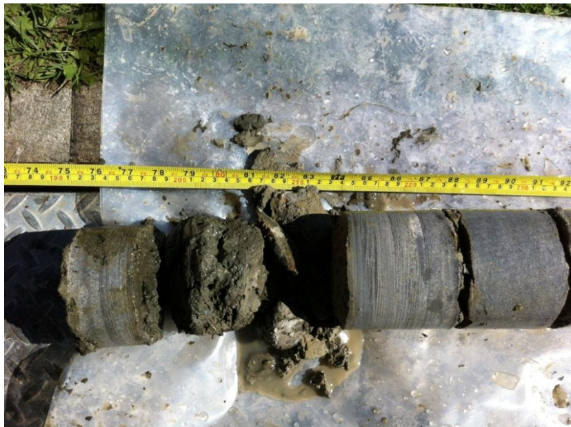
Photograph 10: Layers of clayey silt within the limestone rock
