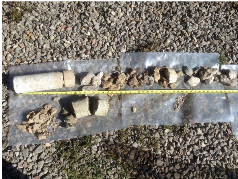
Photograph 6: Corehole CH 13-3 Concrete Cores and Rock Fills or Highly Weathered Rock pieces
