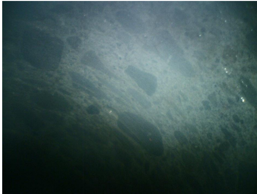
Photograph 1: no cracking or fracture of the pier concrete noted inside the corehole
