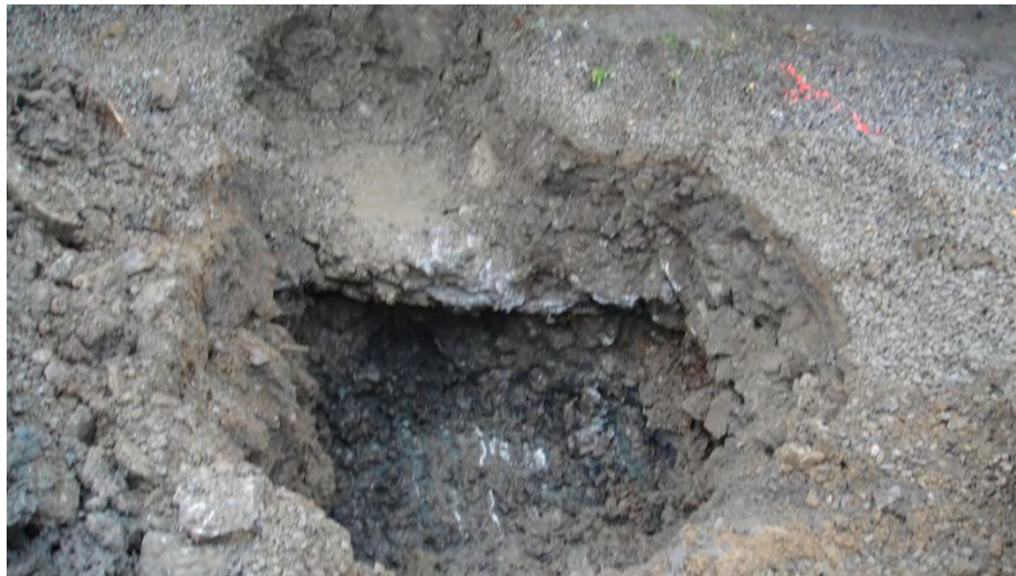
No.36: Photograph of the Test Pit 1. The limestone bedrock exposed at the bottom of the test pit.
