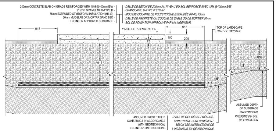
**EXTERIOR GENERATOR PAD - SECTION DETAIL**
