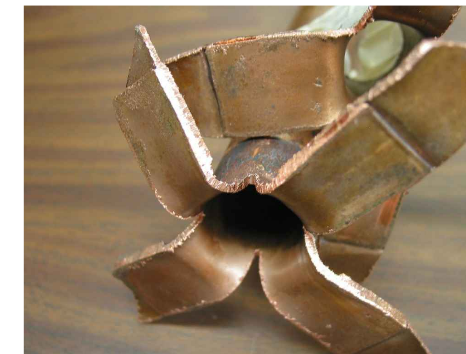
SAMPLE IMAGE OF APPROVED 15% SIL-FOS ARGON PURGED BRAZED PIPING. CONTRACTOR TO PROVIDE TWO SIMILAR SAMPLES FOR ENGINEER APPROVAL.
