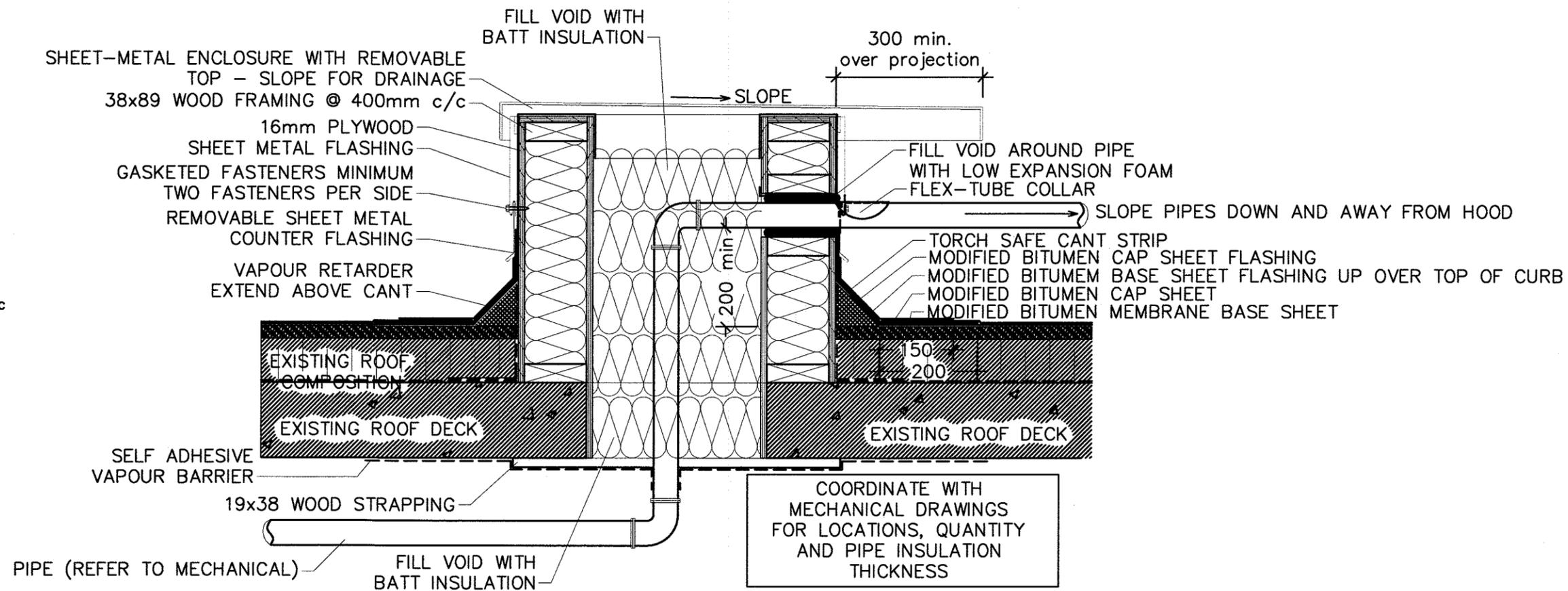
**TYPICAL PIPING ROOF EXIT CURB**
