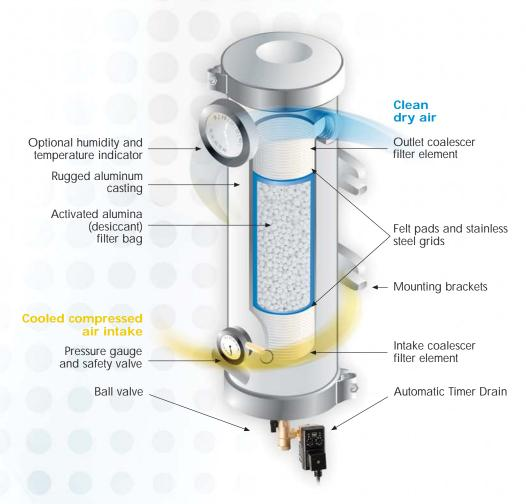
Super-Dry Compressed Air Dryers contain two highly efficient polypropylene coalescer elements at inlet & outlet ports to absorb oil and all solid air particles. Also included, one desiccant bag specifically designed to absorb water vapors and humidity from your compressed air system.
