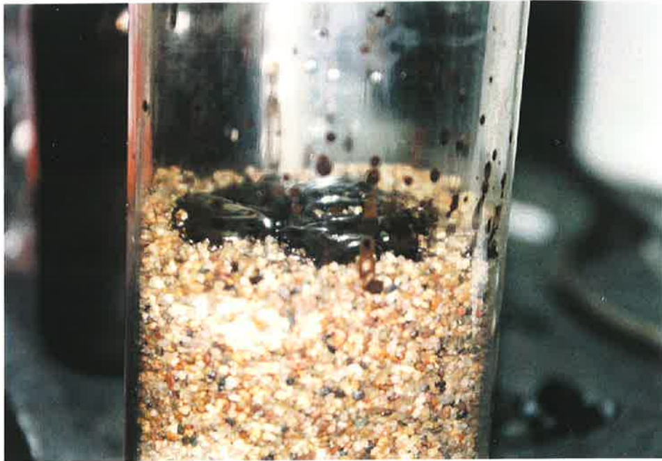
Figure 4. Tarry residue on the surface of a coarse-sand test column. Note the “ropey” nature and viscous consistency.
