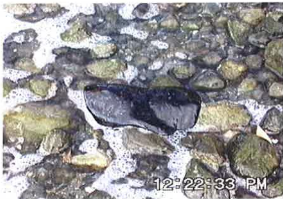
Figure 24 Image capture from video of a coalesced bitumen patty (~20cm in diameter) stranding on pebbles within the swash zone. This patty was not washed off by subsequent swash.
