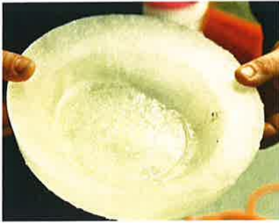
Figure 9 An ice mold prior to filling with coalesced bitumen.
