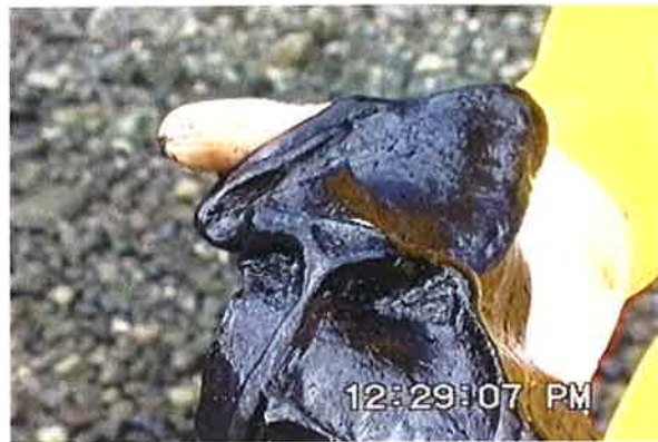
Figure 25 Image capture from video of the same coalesced bitumen patty as shown at left after being peeled off from the pebbles. The patty did not adhere the surface of the pebbles but the pebble casts are clearly visible, indicating that the coalesced bitumen was slowly (~7 minute interval) flowing into the pore spaces of the pebbles.
