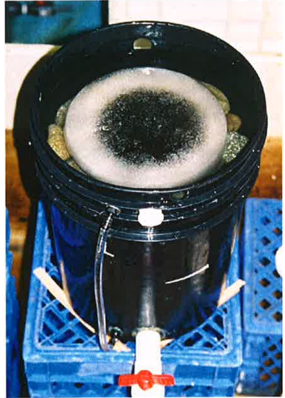
Figure 10 Ice mold and bitumen in inverted position on top of a test column.
