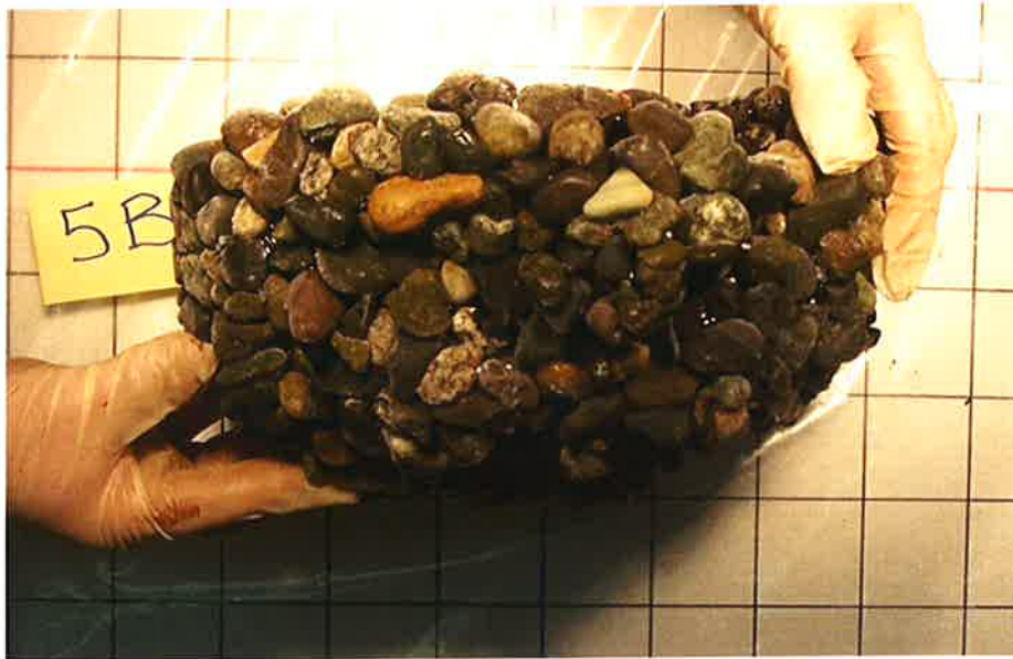
Figure 13 A side-view photo of frozen plug of coalesced bitumen in pebbles. The sediment surface is at the top of the photo and the base or maximum penetration depth at the bottom of the photo. The grid is 5-cm square.
