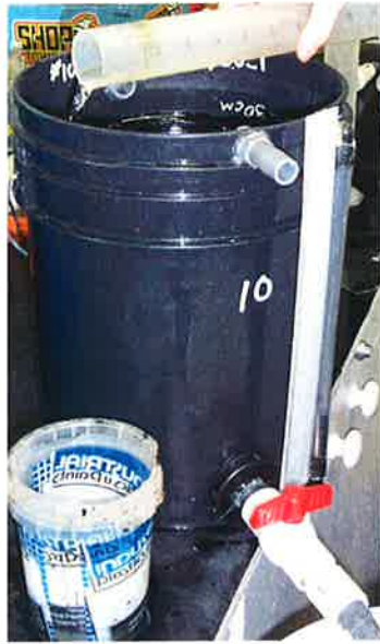
Figure 1 Photograph of pail showing the valve system at the base, the standpipe and the standpipe rule.
